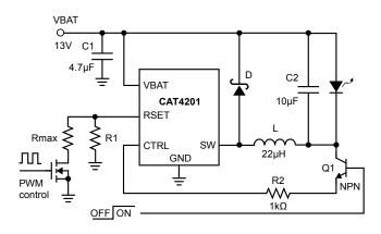
Figure 6. Circuit for PWM on RSET
