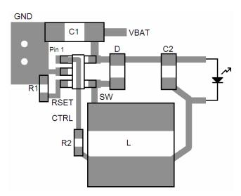
Figure 11. Recommended PCB Layout
