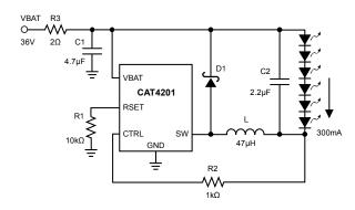
Figure 8. 36V Application with 6 LEDs
