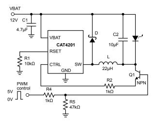
Figure 5. Circuit for PWM on CTRL
