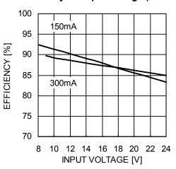
$V_{IN}$  = 13V,  $I_{LED}$  = 300mA, L = 22µH, C<sub>1</sub>= 4.7µF, C<sub>2</sub> = 10µF, T<sub>AMB</sub> = 25°C unless otherwise specified
