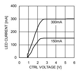
Figure 2. "Dropout" configured LED Current (as shown in Typical Application on page 1)
