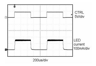
Figure 3. PWM at 1kHz on CTRL Pin
