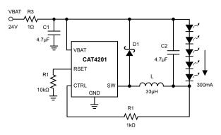
Figure 7. 24V Application with 5 LEDs
