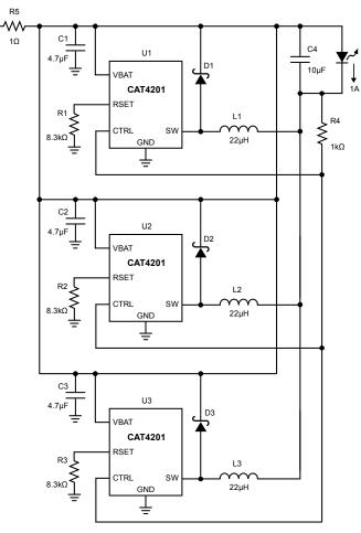
Figure 9. Three CAT4201 in Parallel for 1A LED
