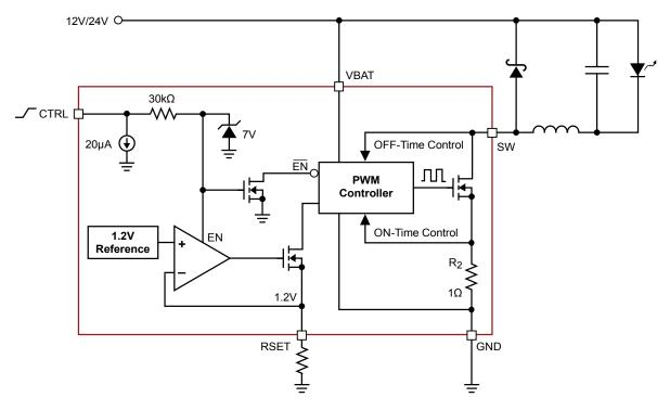
Figure 1. CAT4201 Simplified Block Diagram
