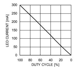
Figure 4. LED Current vs. Duty Cycle
