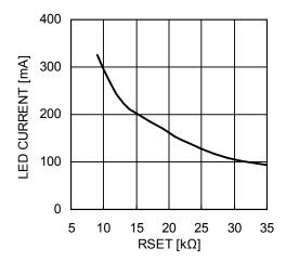
$V_{IN}$  = 13V,  $I_{LED}$  = 300mA, L = 22µH, C<sub>1</sub>= 4.7µF, C<sub>2</sub> = 10µF, T<sub>AMB</sub> = 25°C unless otherwise specified
