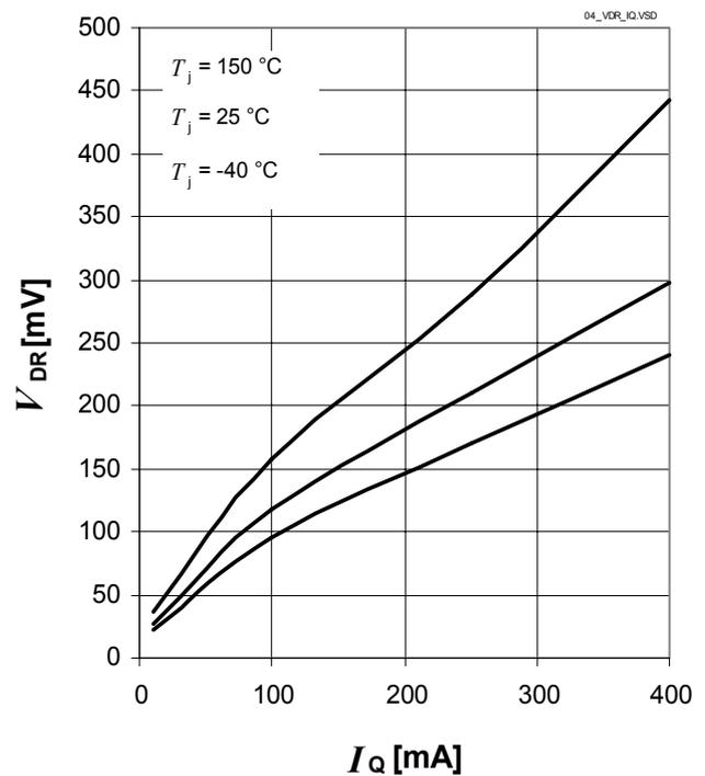
**Dropout Voltage  $V_{dr}$  versus Junction Temperature**
