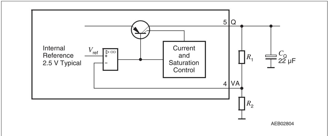
**Figure 4 External Components at Output for Variable Voltage Regulator**
