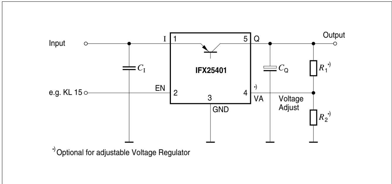
Figure 3 Application Diagram
