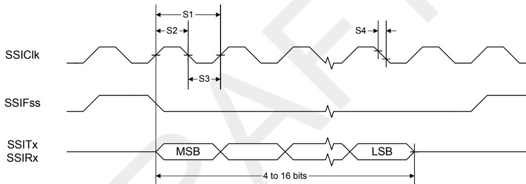
Figure 21-5. SSI Timing for MICROWIRE Frame Format (FRF=10), Single Transfer
