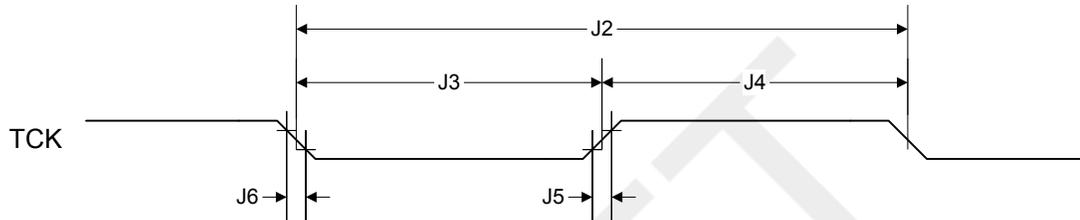
Figure 21-8. JTAG Test Access Port (TAP) Timing
