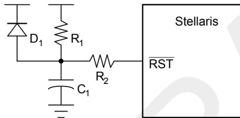
The  $R_1$  and  $C_1$  components define the power-on delay. The  $R_2$  resistor mitigates any leakage from the  $\overline{RST}$  input. The diode ( $D_1$ ) discharges  $C_1$  rapidly when the power supply is turned off.
