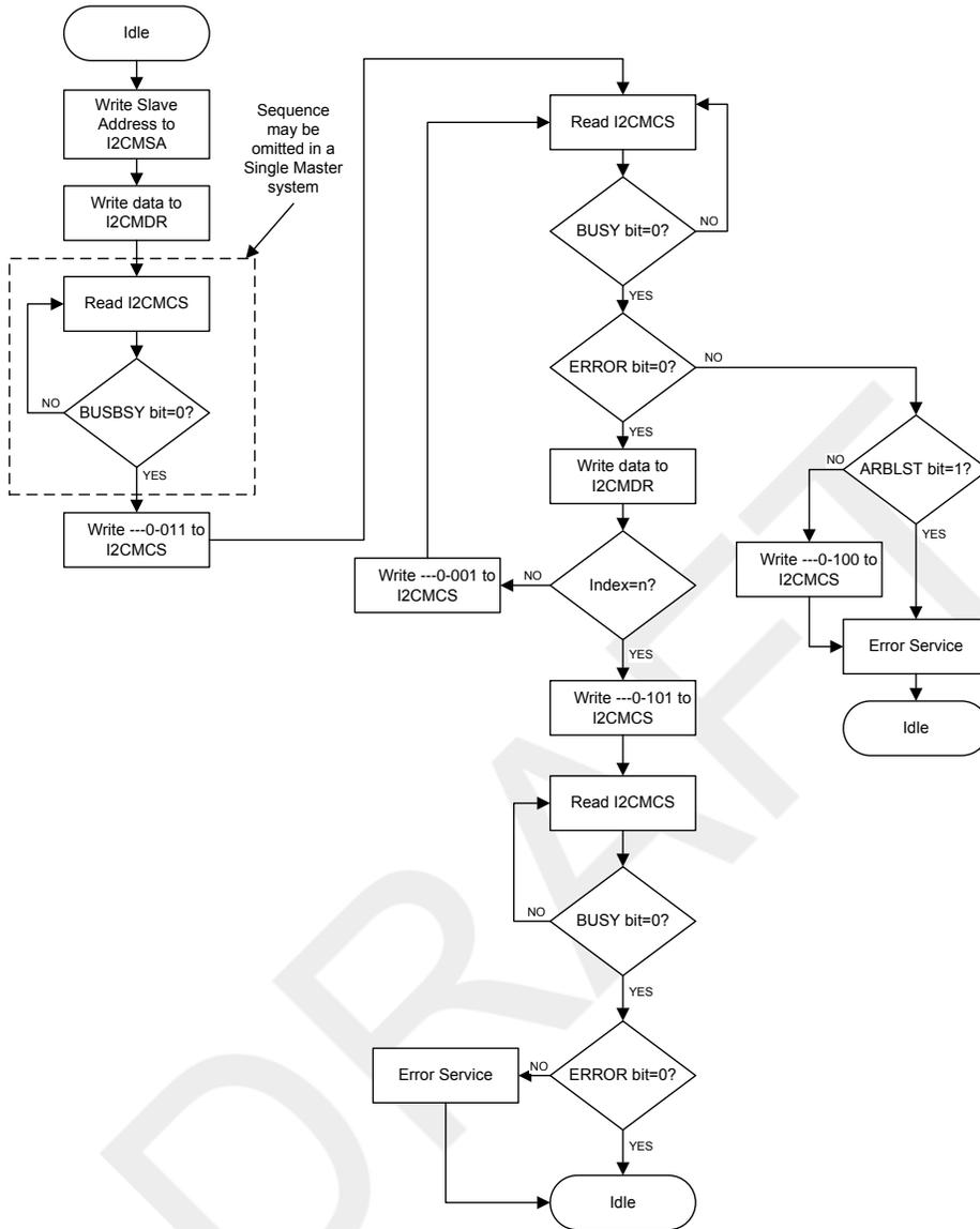
Figure 14-10. Master Burst RECEIVE
