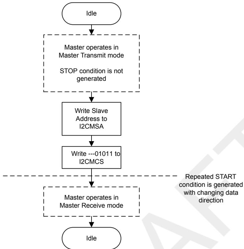
Figure 14-12. Master Burst SEND after Burst RECEIVE
