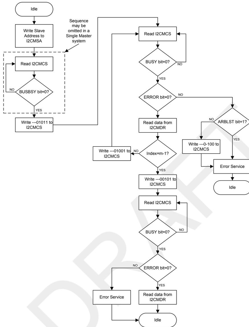
Figure 14-11. Master Burst RECEIVE after Burst SEND
