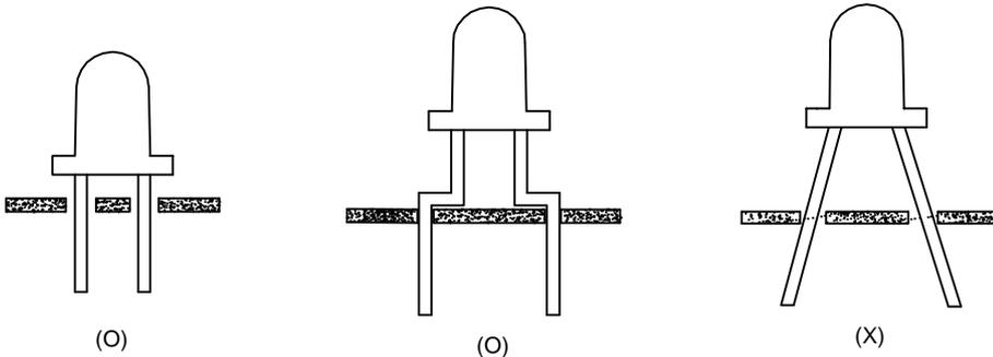
2. The LED lamps are designed for high-density mounting and have a structure which can alleviate mechanical stress due to clinching . Nevertheless , take care to avoid the occurrence of residual mechanical stress due to clinching .
