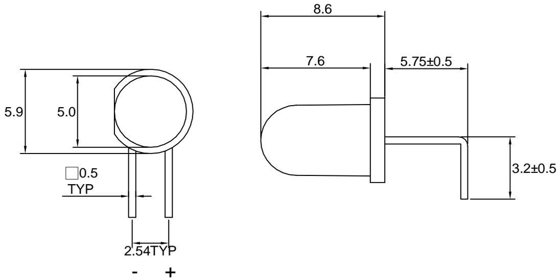
Note : 1.All dimension are in millimeter tolerance is  $\pm 0.25\text{mm}$  unless otherwise noted.
