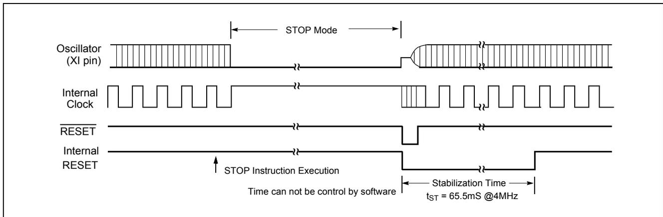
Figure 19-6 Timing of STOP Mode Release by Reset
