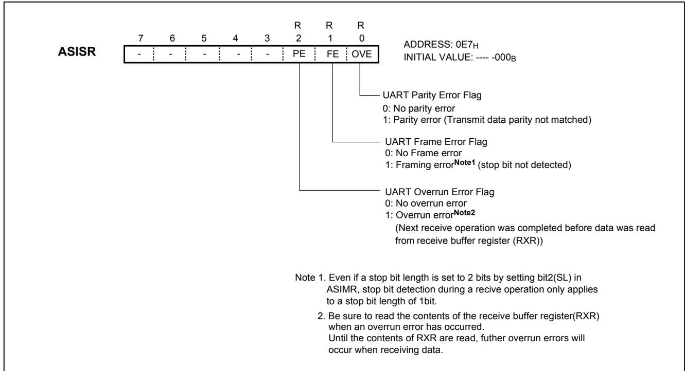
**Figure 16-4 Asynchronous Serial Interface Status Register (ASISR) Format**
