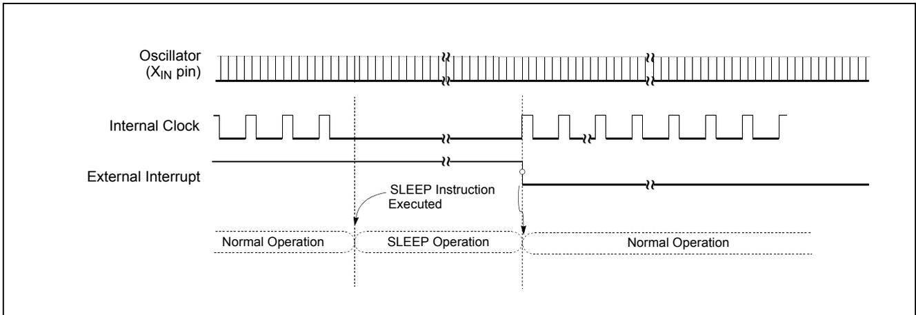
Figure 19-2 SLEEP Mode Release Timing by External Interrupt
