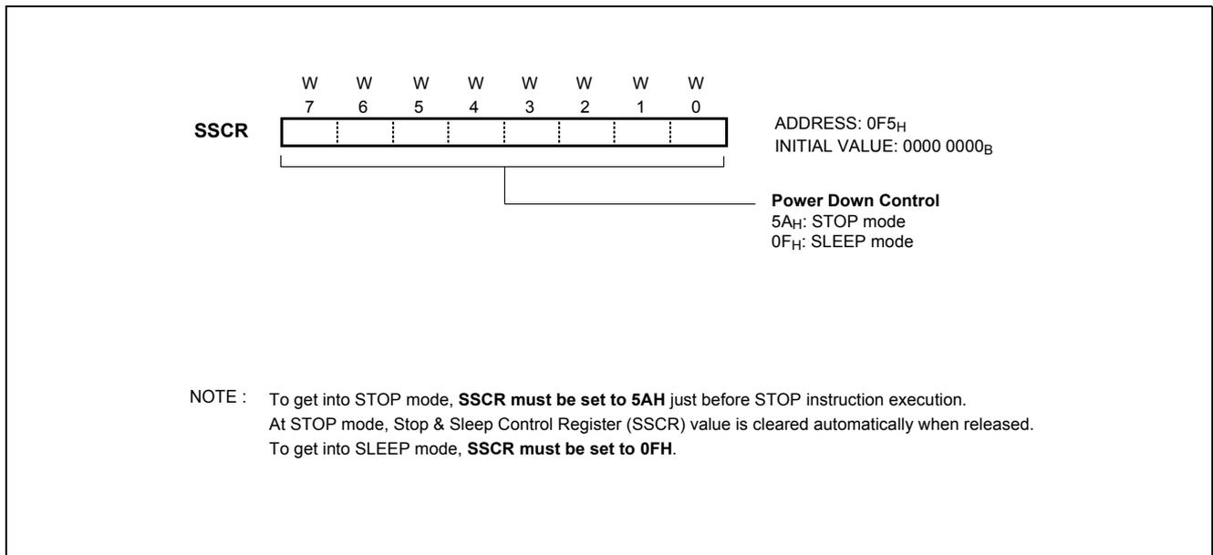
Figure 19-1 STOP and SLEEP Control Register
