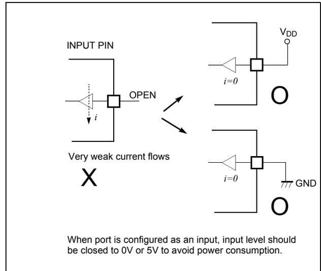
Figure 19-9 Application Example of Unused Input Port
