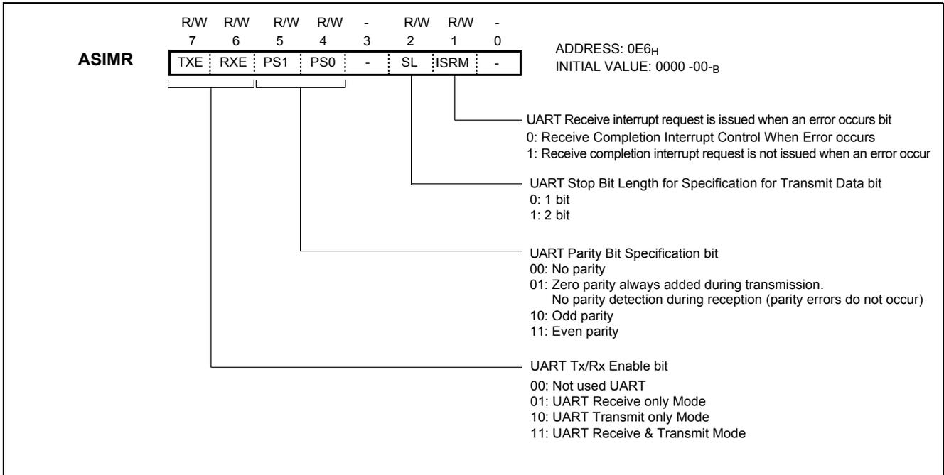
Figure 16-3 Asynchronous Serial Interface Mode register (ASIMR) Format
