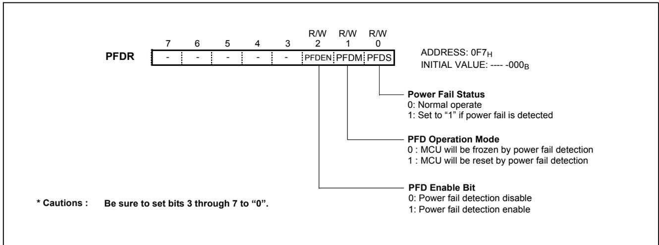
Figure 21-1 Power Fail Voltage Detector Register
