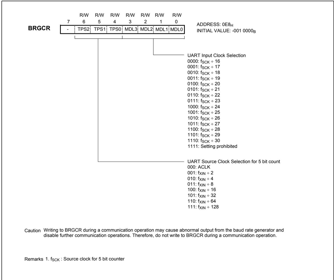
**Figure 16-5 Baud Rate Generator Control Register (BRGCR) Format**
