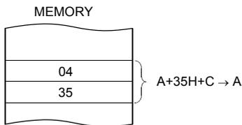
When G-flag is 1, then RAM address is defined by 16-bit address which is composed of 8-bit RAM paging register (RPR) and 8-bit immediate data.
