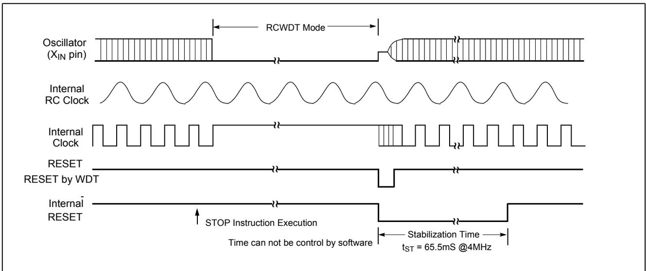
Figure 19-8 Internal RC-WDT Mode Releasing by Reset
