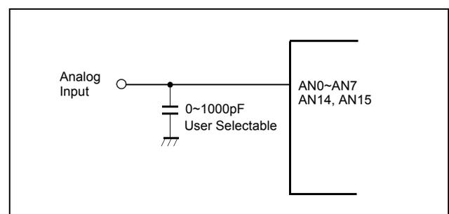
Figure 14-2 Analog Input Pin Connecting Capacitor
