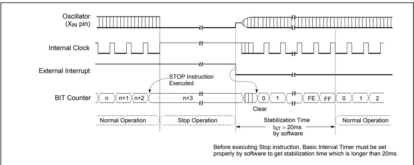
Figure 19-5 STOP Mode Release Timing by External Interrupt
