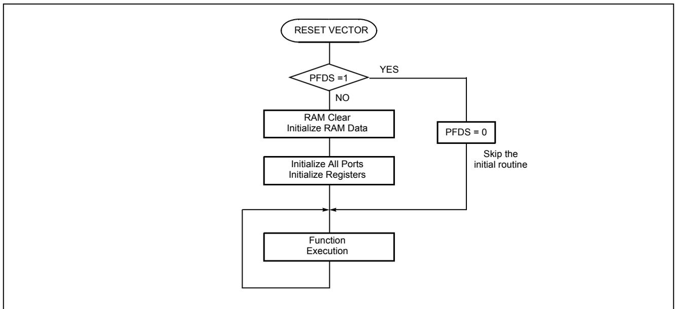
Figure 21-2 Example S/W of Reset flow by Power fail
