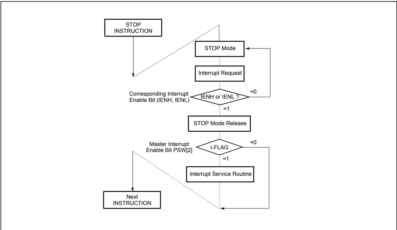
Figure 19-4 STOP Releasing Flow by Interrupts
