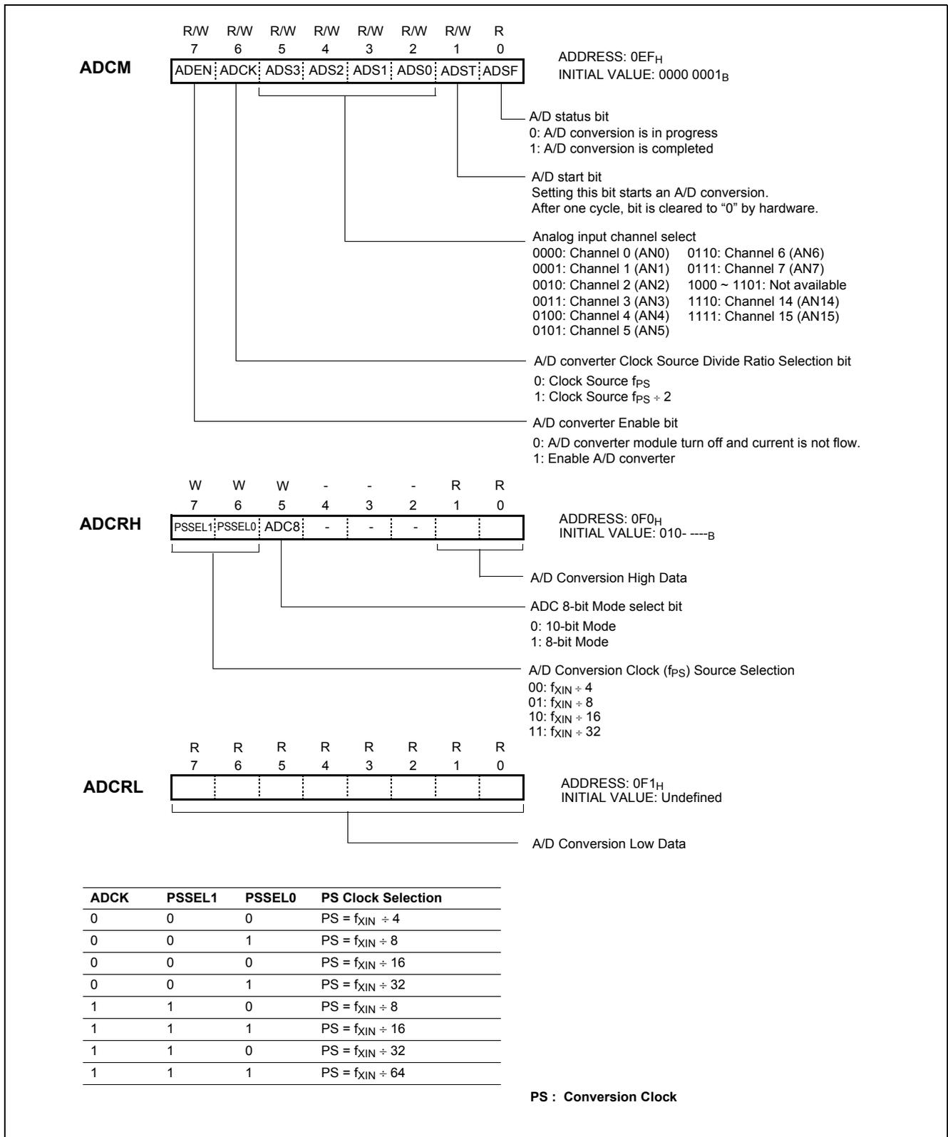
Figure 14-4 A/D Converter Control & Result Register
