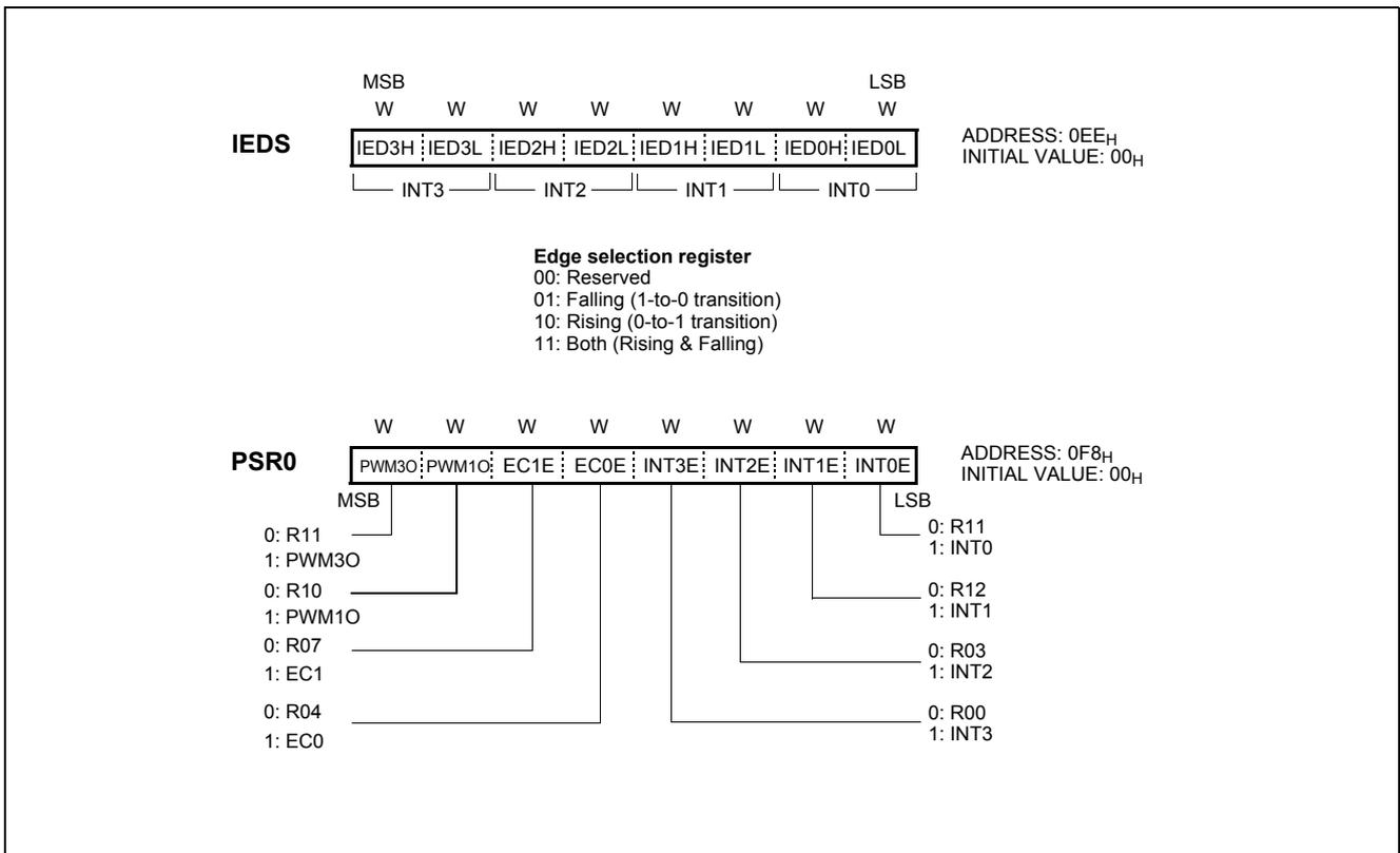
Figure 18-9 IEDS register and Port Selection Register PSR0
