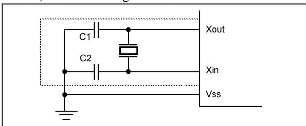
Figure 10-2 Oscillator Connections
