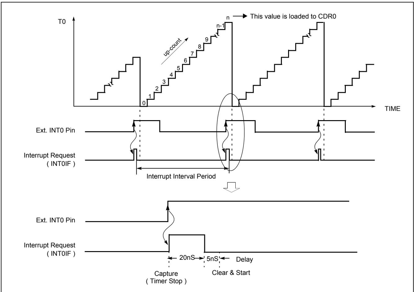
Figure 13-13 Input Capture Operation of Timer 0 Capture mode
