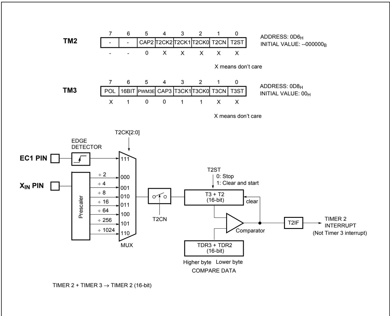
Figure 13-10 16-bit Timer/Counter for Timer 2, 3
