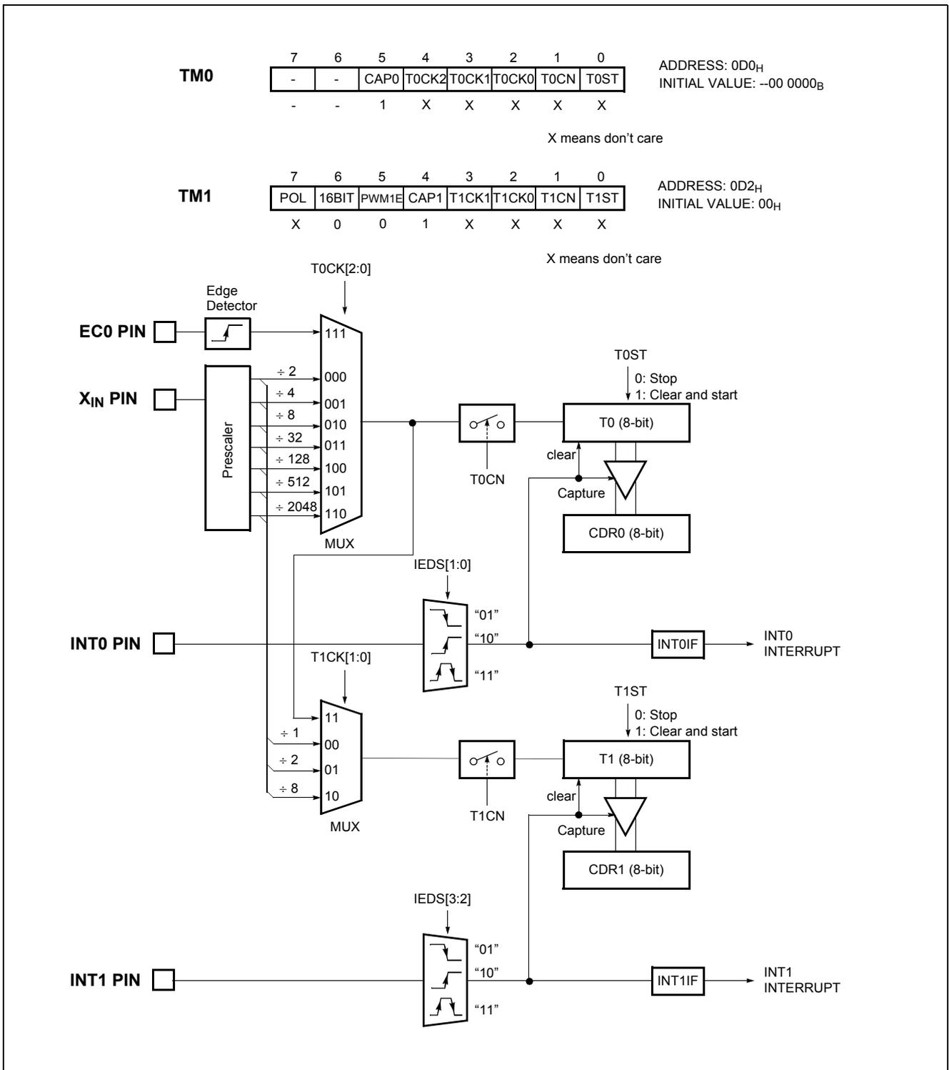
Figure 13-11 8-bit Capture Mode for Timer 0, 1
