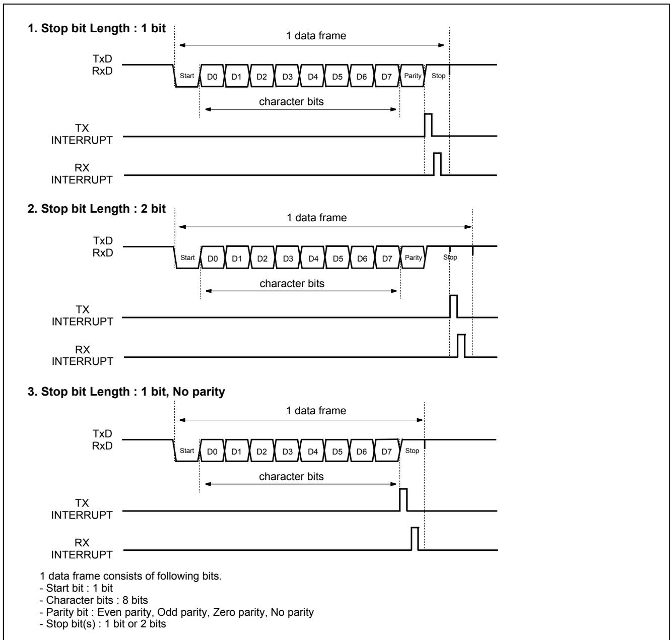
Figure 16-6 UART data format and interrupt timing diagram
