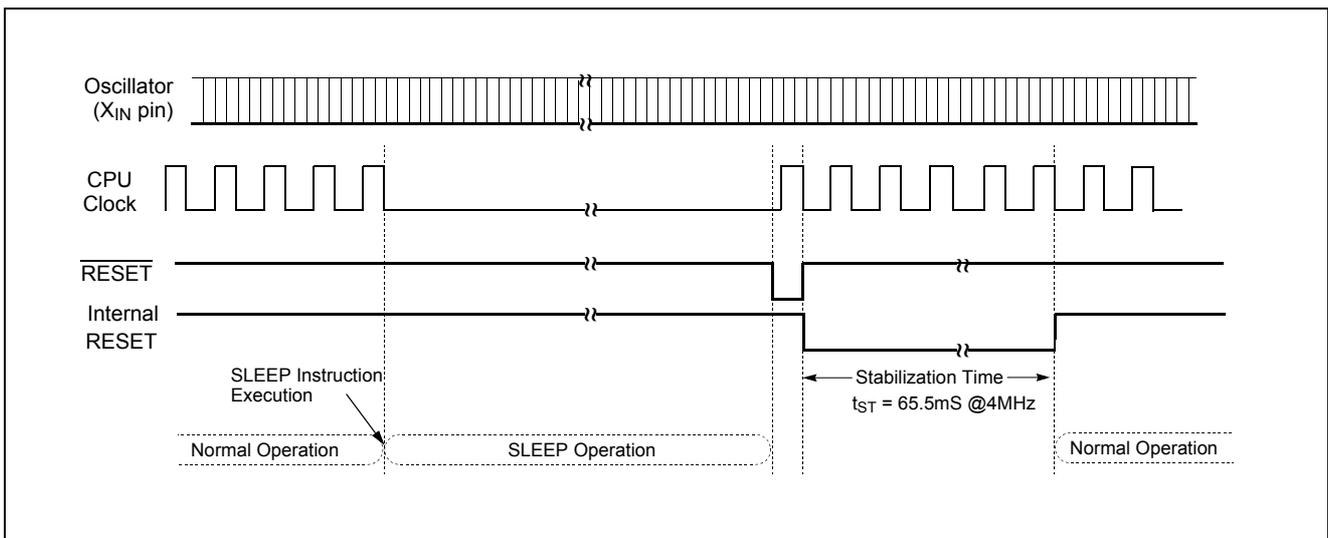
Figure 19-3 Timing of SLEEP Mode Release by Reset
