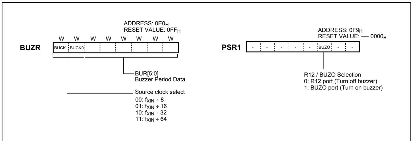
Figure 17-2 Buzzer Register & PSR1
