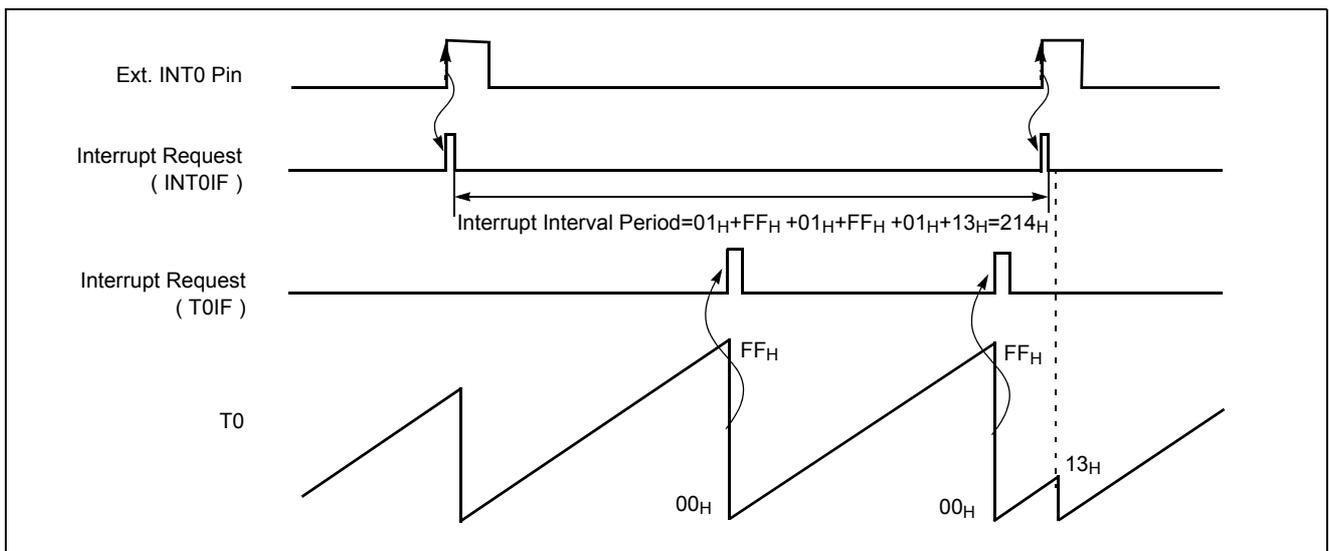
Figure 13-14 Excess Timer Overflow in Capture Mode
