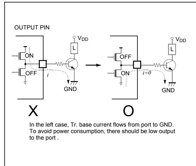
Figure 19-10 Application Example of Unused Output Port
