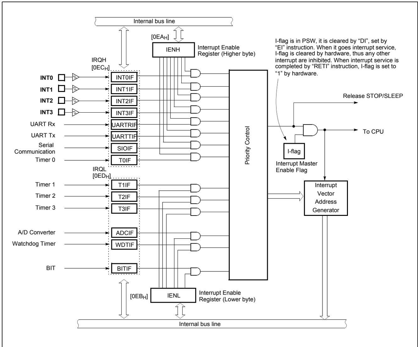
Figure 18-1 Block Diagram of Interrupt
