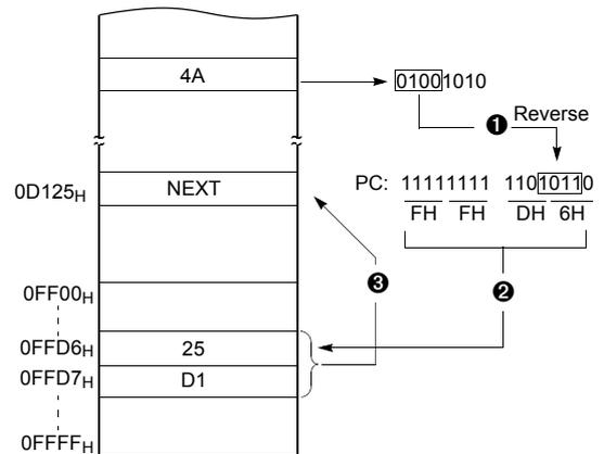
Example: The usage software example of Vector address for MC80F0204.
