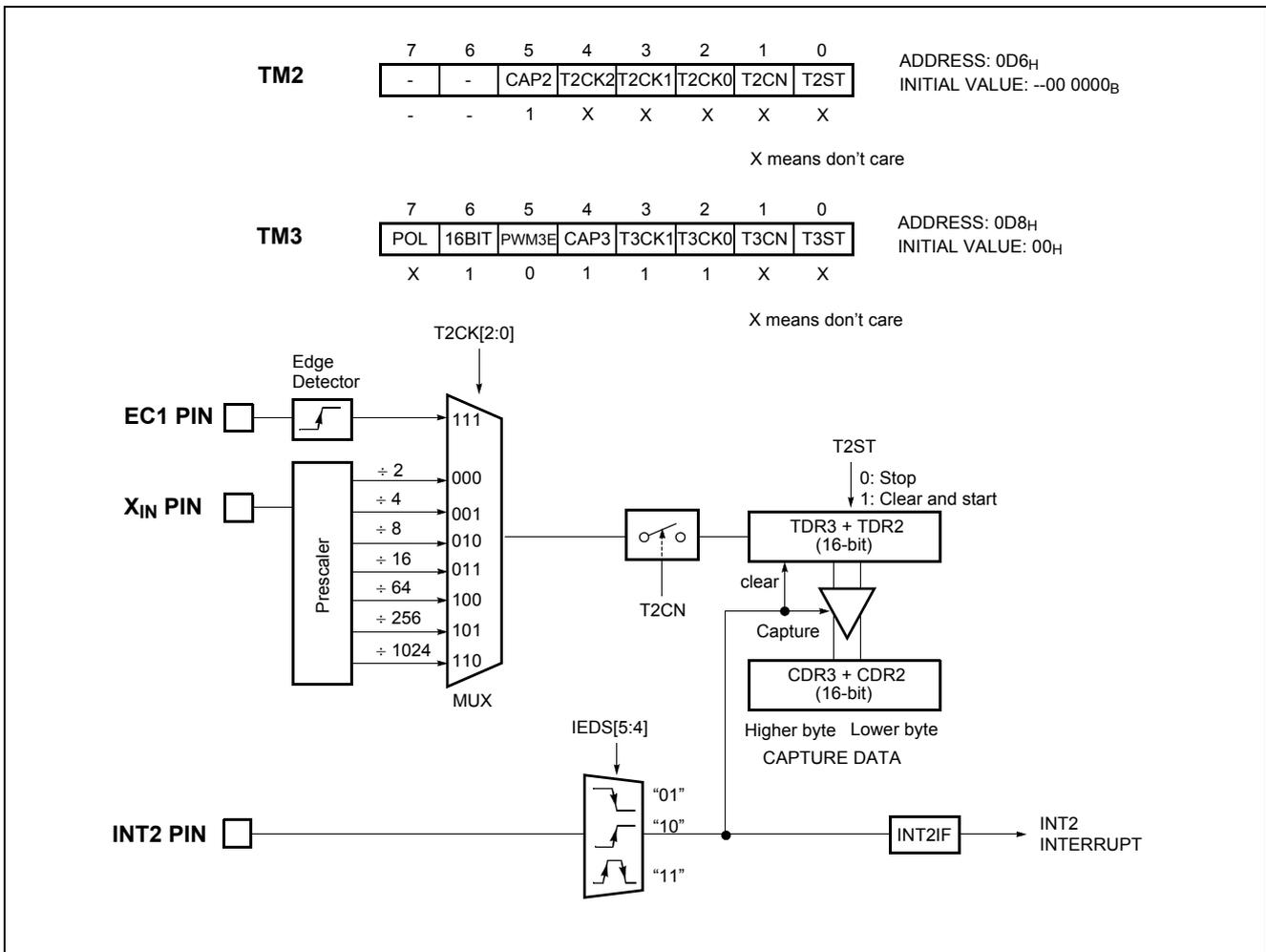
Figure 13-16 16-bit Capture Mode of Timer 2, 3
