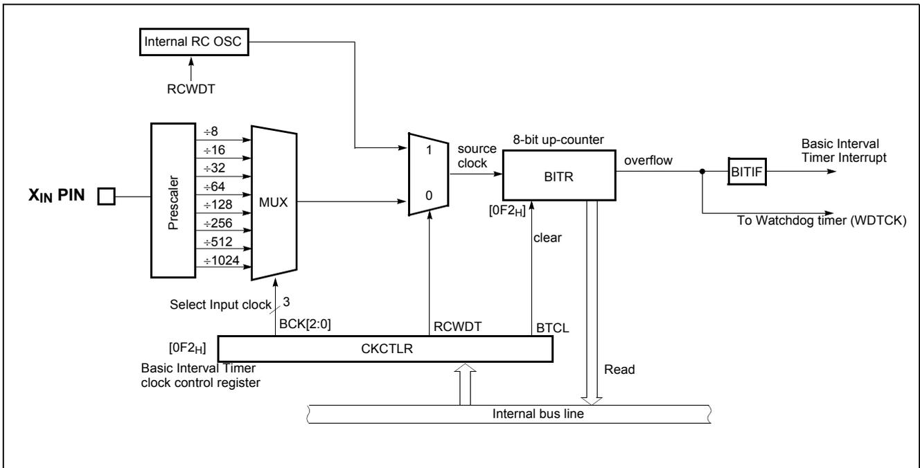
Figure 11-1 Block Diagram of Basic Interval Timer
