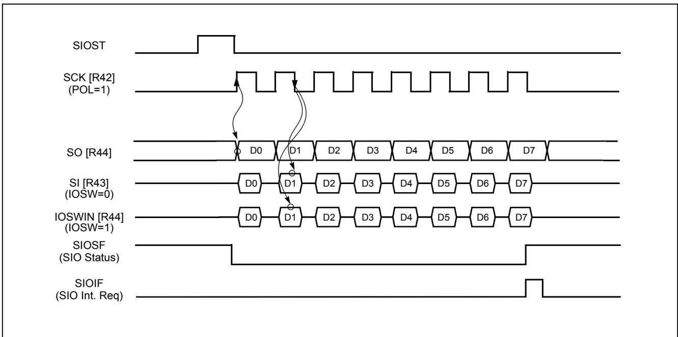
Figure 15-4 Serial I/O Timing Diagram at POL=1
