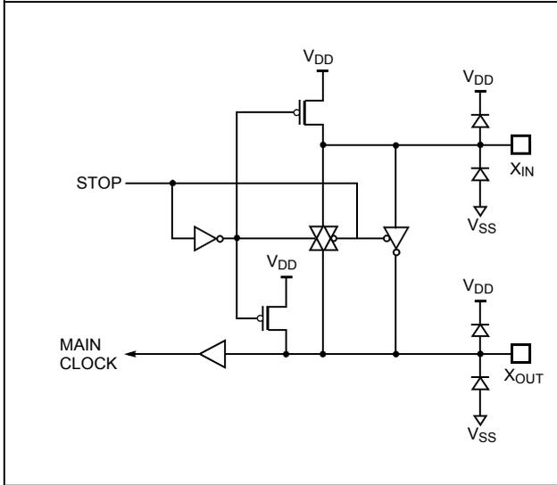
**X<sub>IN</sub>, X<sub>OUT</sub> (External RC or R oscillation)**
