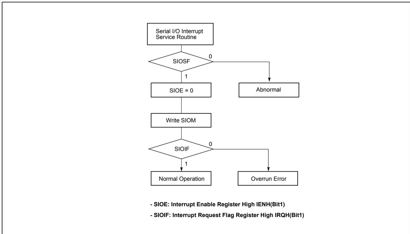
Figure 15-5 Serial IO Method to Test Transmission
