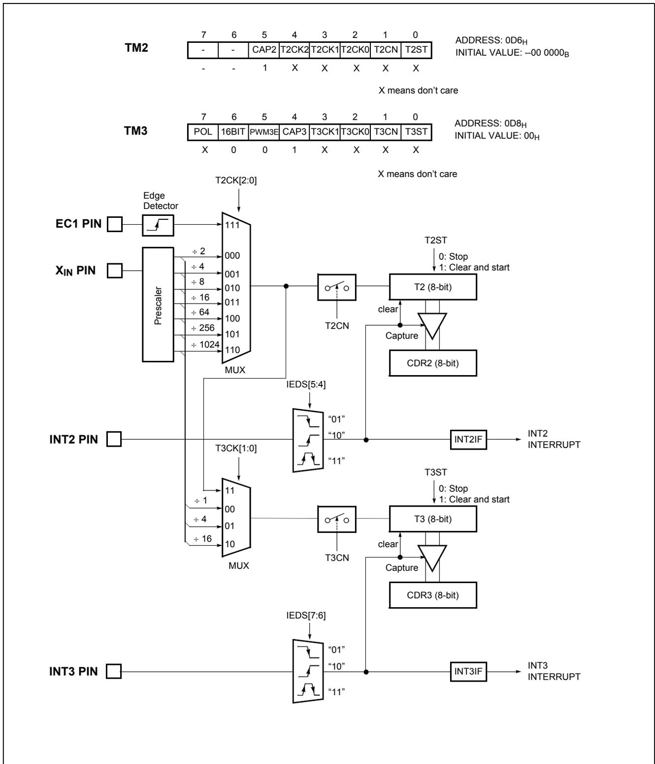
Figure 13-12 8-bit Capture Mode for Timer 2, 3
