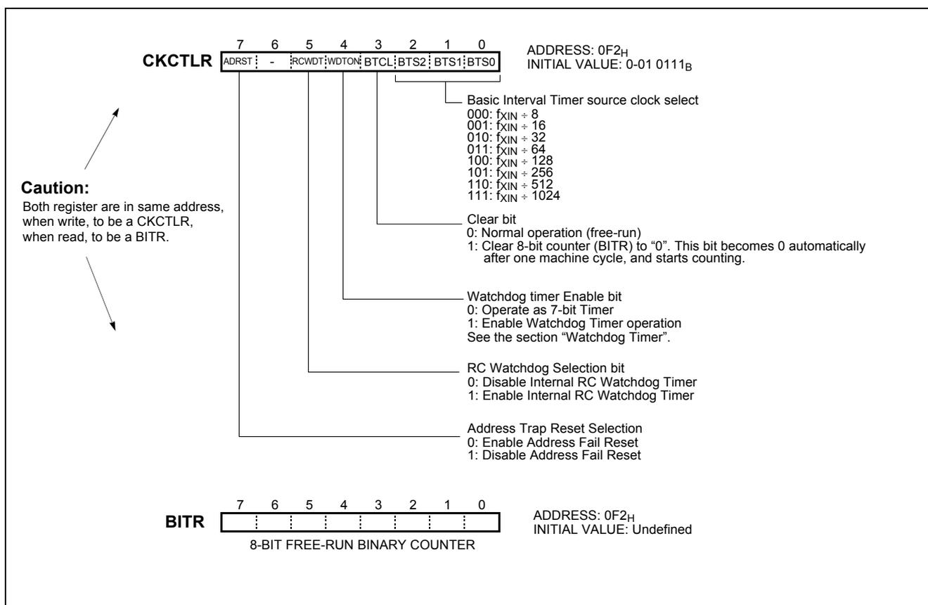
Figure 11-2 BITR: Basic Interval Timer Mode Register
