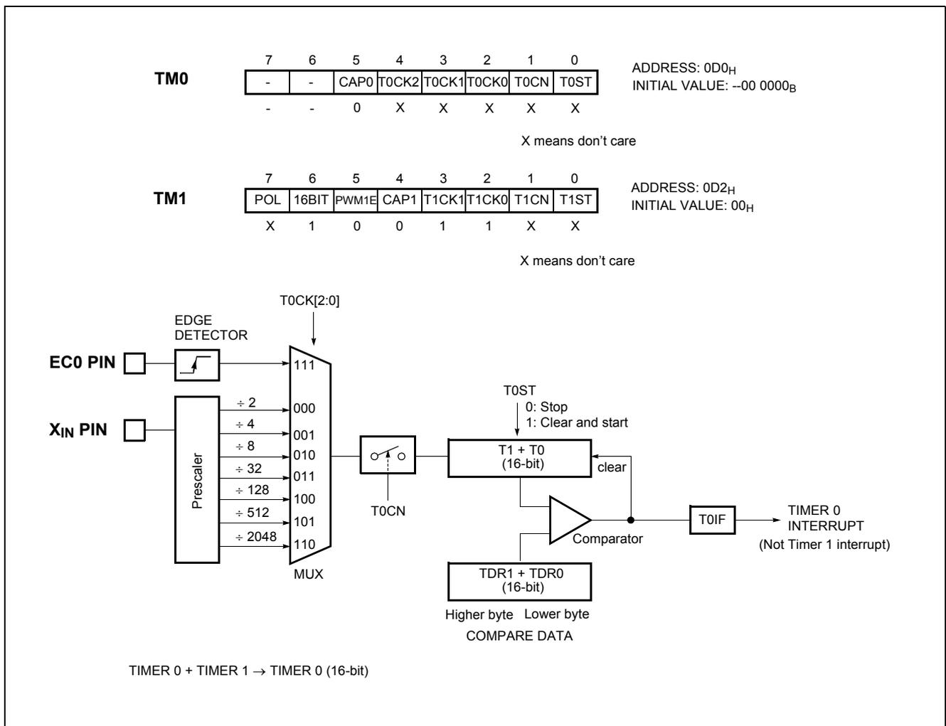
Figure 13-9 16-bit Timer/Counter for Timer 0, 1
