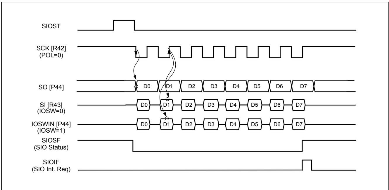
Figure 15-3 Serial I/O Timing Diagram at POL=0
