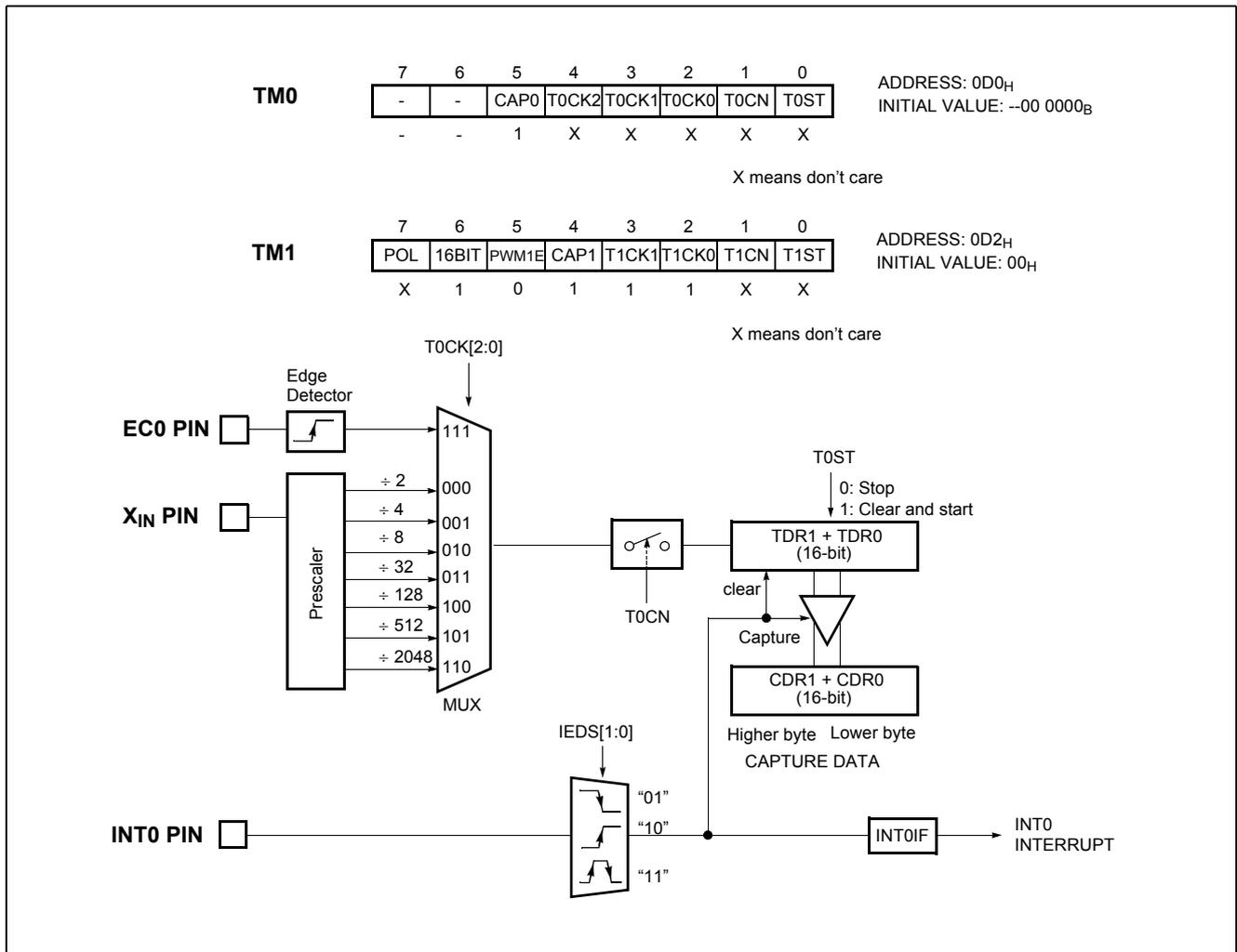
Figure 13-15 16-bit Capture Mode of Timer 0, 1
