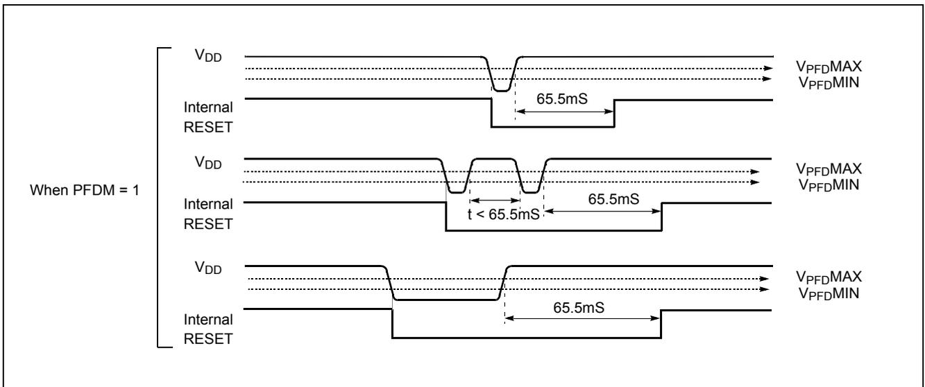
Figure 21-3 Power Fail Processor Situations (at 4MHz operation)
