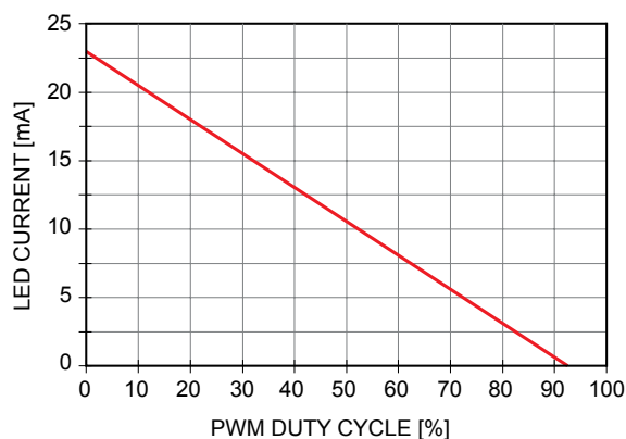
Figure 3. Filtered PWM Dimming [0V to 2.5V]
