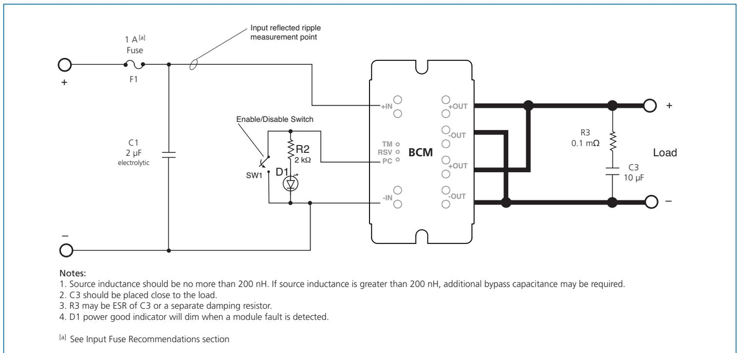
Figure 15 — VI BRICK BCM test circuit
