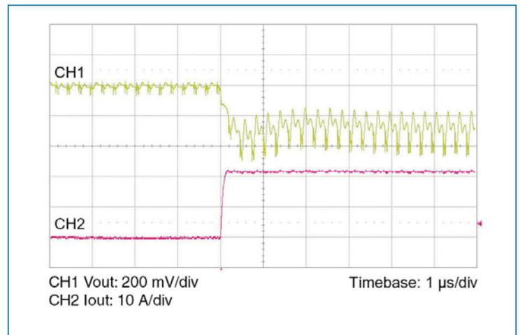
Figure 10 — 0-21.8 A load step with 2  $\mu\text{F}$  input capacitor and no output capacitor.
