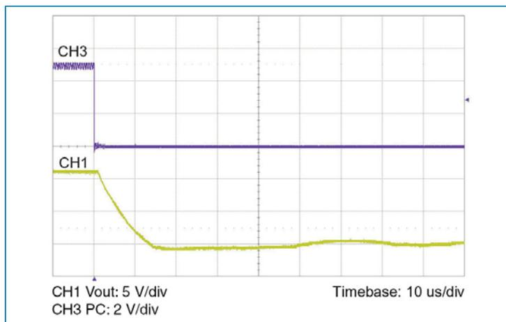
Figure 12 —  $V_{OUT}$  at full load vs. PC disable
