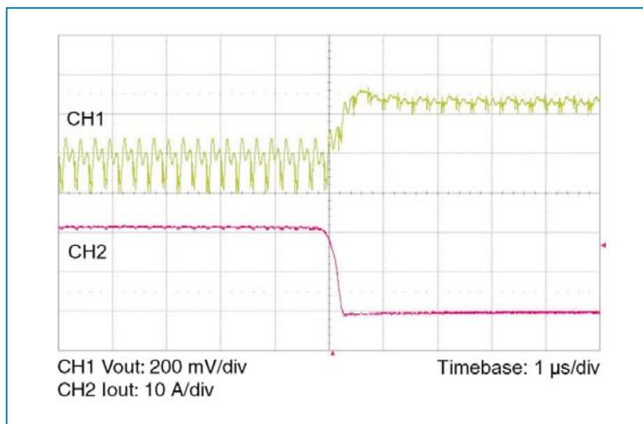
Figure 11 — 21.8-0 A load step with 2  $\mu\text{F}$  input capacitor and no output capacitor.
