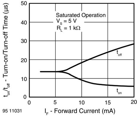
Fig. 12 - Turn-on/turn-off Time vs. Forward Current
