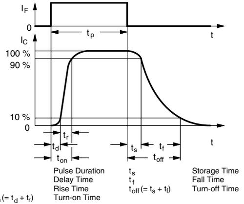
Fig. 3 - Switching Times
