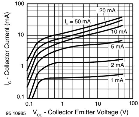
Fig. 9 - Collector Current vs. Collector Emitter Voltage
