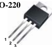
1. Gate 2. Drain 3. Source
