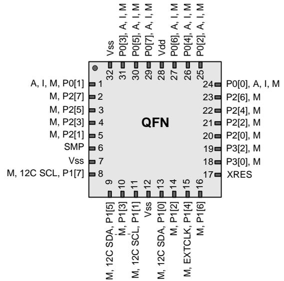
**Table 4. 32-Pin Part Pinout (QFN\*)**
