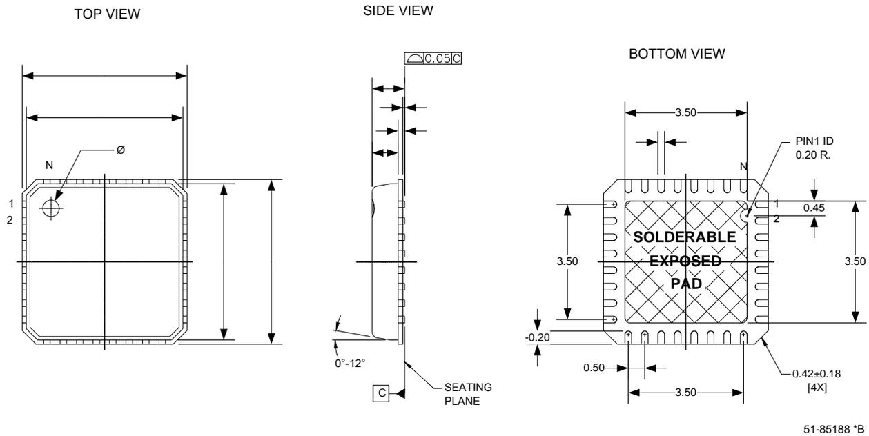
Figure 19. 32-Pin QFN (5 x 5 mm) (Sawn)
