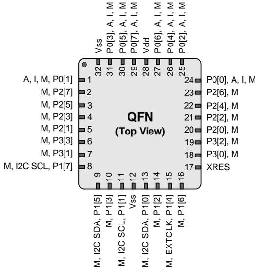
Figure 7. CY7C60333-LFXC 32-Pin Device
