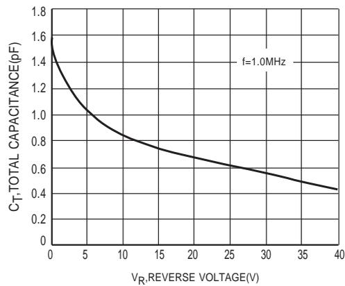
Figure 3 Typical Capacitance
