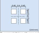
The recommended thickness of the screen mask for soldering is between 80 and 130 $\mu\text{m}.$  The hole size of the screen mask should be same as the recommended land pattern or smaller.
