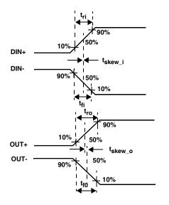
FIGURE 6A. MEASUREMENT POINTS
