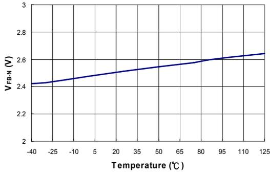
**Figure 13. Green-Mode Entry FB Voltage (V<sub>FB-N</sub>) vs. Temperature**
