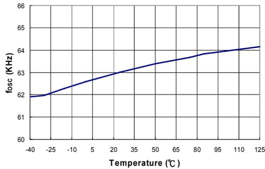
**Figure 11. Center Frequency (f<sub>OSC</sub>) vs. Temperature**
