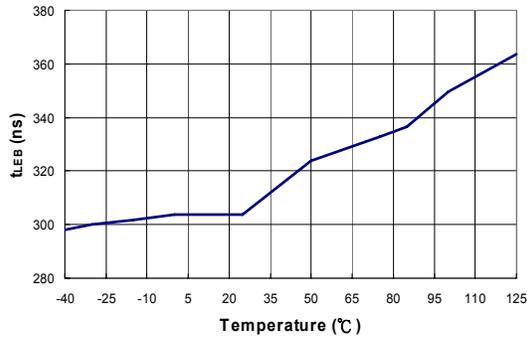
**Figure 15. Leading-Edge Blanking Time (t<sub>LEB</sub>) vs. Temperature**
