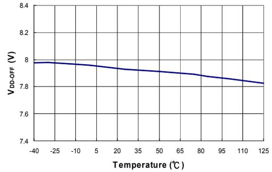
**Figure 8. Turn-off Threshold Voltage (V<sub>DD-OFF</sub>) vs. Temperature**
