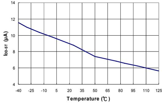
**Figure 9. Startup Current (I<sub>DD-ST</sub>) vs. Temperature**
