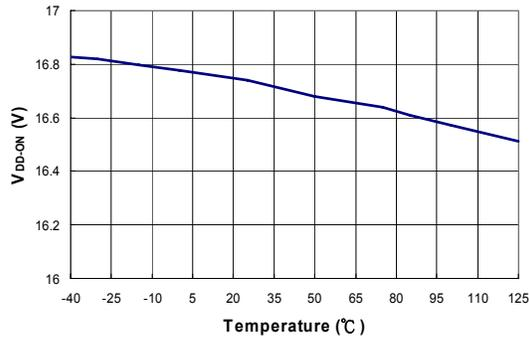
**Figure 7. Turn-on Threshold Voltage (V<sub>DD-ON</sub>) vs. Temperature**
