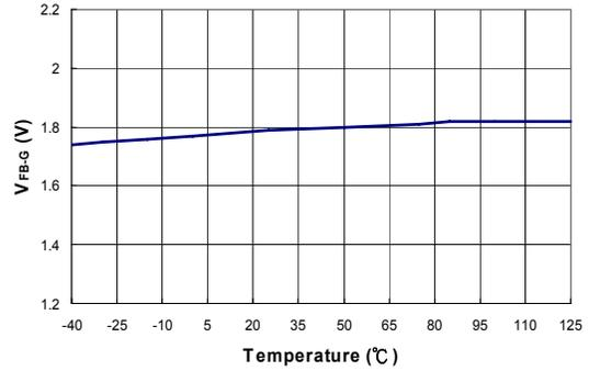
**Figure 14. Green-Mode Ending FB Voltage (V<sub>FB-G</sub>) vs. Temperature**
