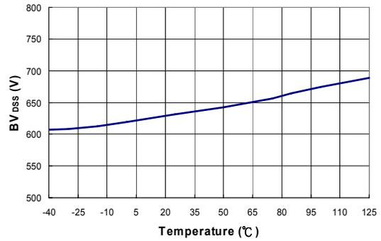
**Figure 16. Drain-Source Breakdown Voltage (BV<sub>DSS</sub>) vs. Temperature**
