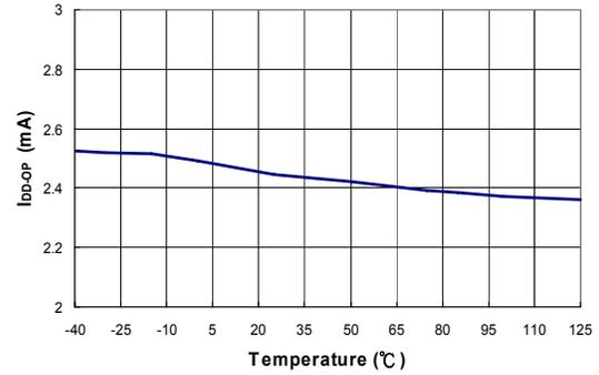
**Figure 10. Operating Supply Current (I<sub>DD-OP</sub>) vs. Temperature**
