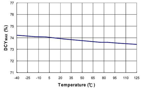
**Figure 12. Maximum Duty Cycle (DCY<sub>MAX</sub>) vs. Temperature**
