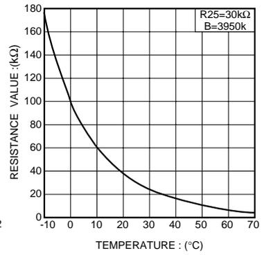
Fig. 3 Thermistor curve
