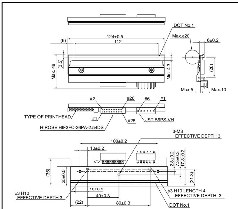
Note: No heat history control function inside the thermal printhead. External heat history control is required for high speed printing.
