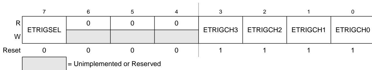
Figure 4-4. ATD Control Register 1 (ATDCTL1)
