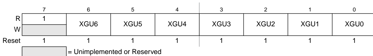
Figure 17-18. RAM XGATE Upper Boundary Register (RAMXGU)
