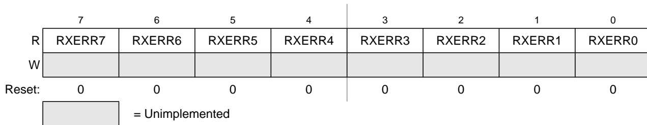
Figure 10-18. MSCAN Receive Error Counter (CANRXERR)
