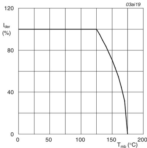
$$I_{der} = \frac{I_D}{I_{D(25^\circ\text{C})}} \times 100\%$$
