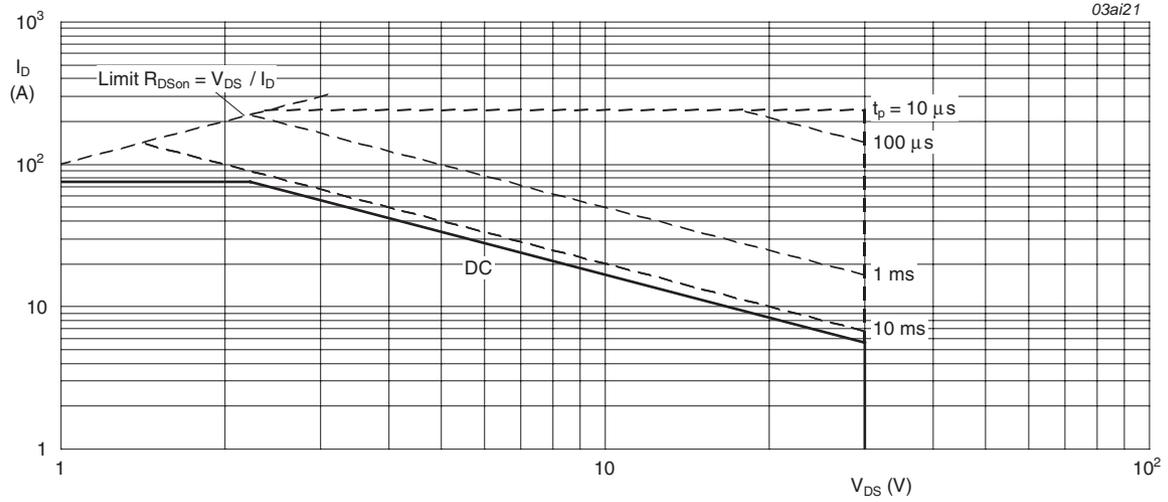
$T_{mb} = 25^\circ C; I_{DM}$  is single pulse;  $V_{GS} = 10V$
