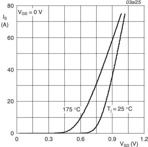
$T_j = 25^\circ C$  and  $175^\circ C; V_{GS} = 0V$
