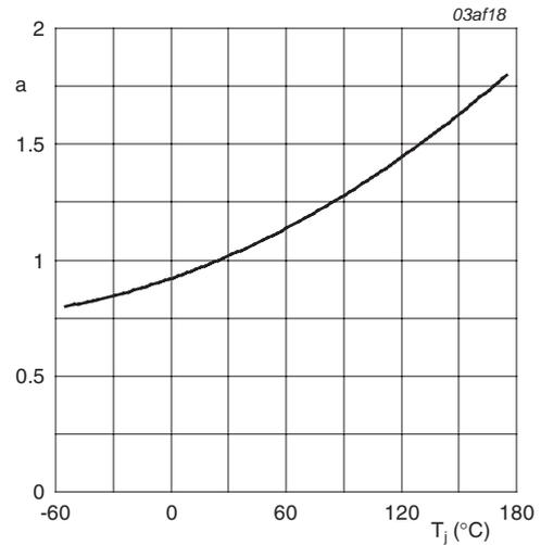
$$a = \frac{R_{DSon}}{R_{DSon(25^\circ\text{C})}}$$
