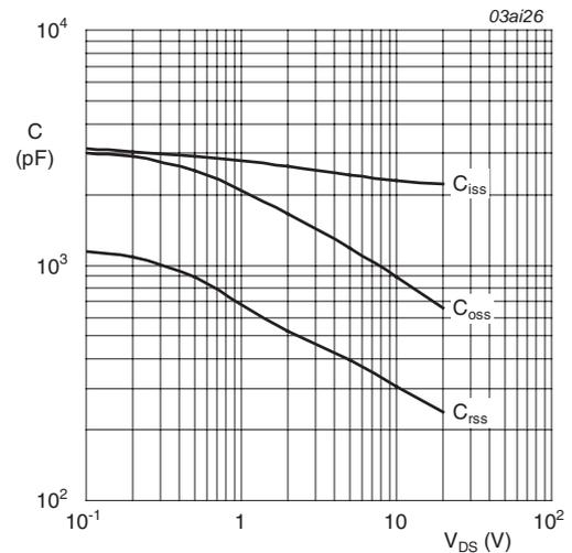
$V_{GS} = 0\text{ V}; f = 1\text{ MHz}$
