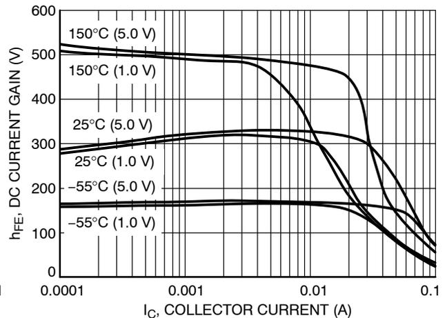
**Figure 2. DC Current Gain vs. Collector Current**
