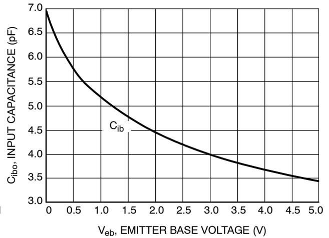
**Figure 6. Input Capacitance**
