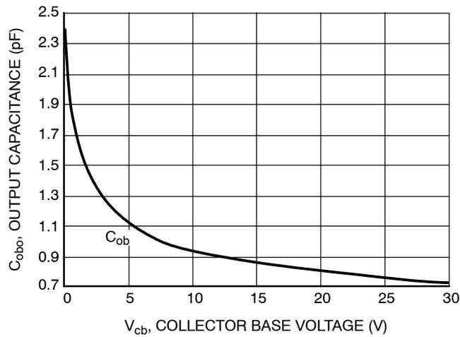
**Figure 7. Output Capacitance**
