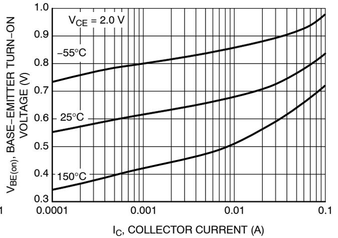
**Figure 4. Base Emitter Turn-On Voltage vs. Collector Current**
