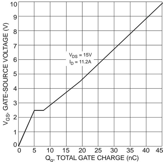
Fig. 11 Gate-Source Voltage vs. Total Gate Charge
