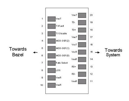
Figure 3 Transceiver pin descriptions
