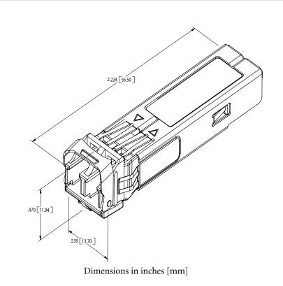
An eye-safe, cost effective serial transceiver, the PLRXPL-VI-S24-22 features a small, low power, pluggable package that manufacturers can upgrade in the field, adding bandwidth incrementally. The robust mechanical design features a unique all-metal housing that provides superior EMI shielding.
