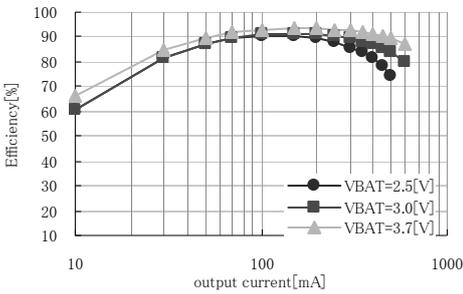
Fig.1 Output current - Efficiency characteristic (5.015[V] Output voltage setting)
