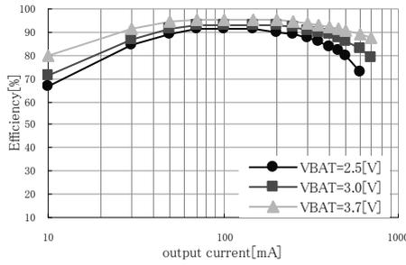
Fig.2 Output current - Efficiency characteristic (4.2[V] Output voltage setting)
