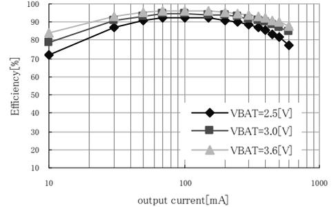
Fig.3 Output current - Efficiency characteristic (3.6[V] Output voltage setting)
