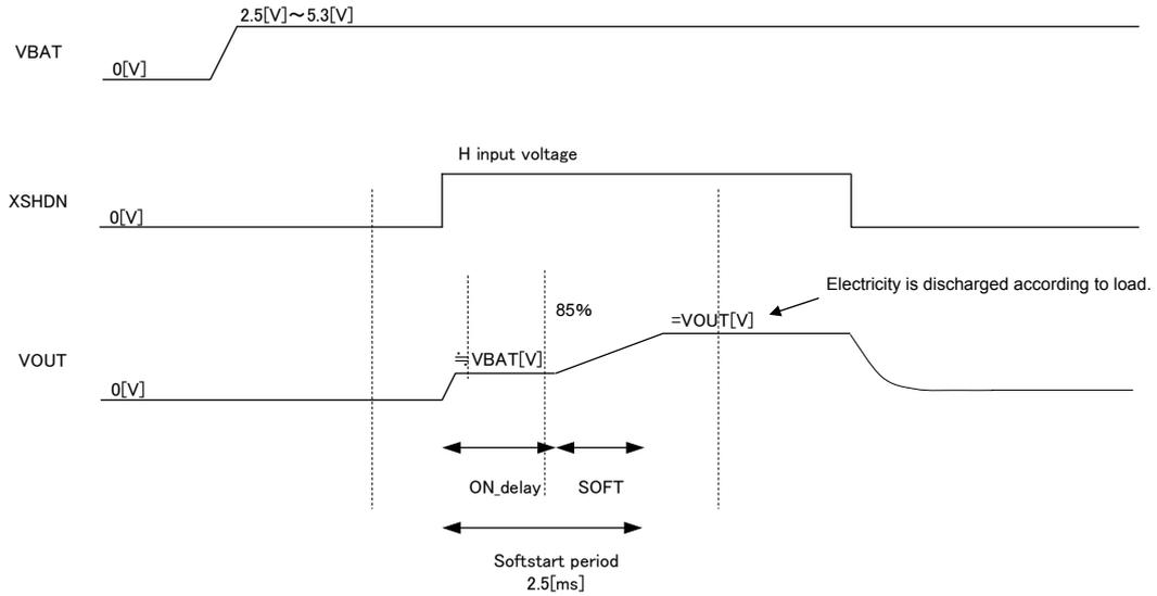
Fig.14 DC/DC converter start wave form
