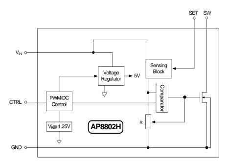
Figure 2: AP8802H Block Diagram
