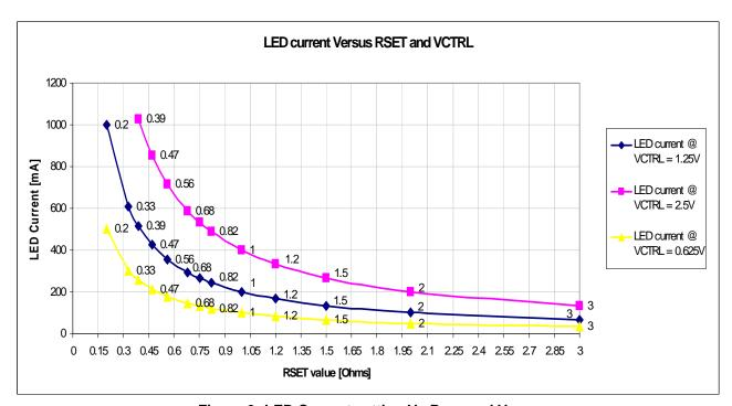
Figure 3: LED Current setting Vs R<sub>SET</sub> and V<sub>CTRL</sub>
