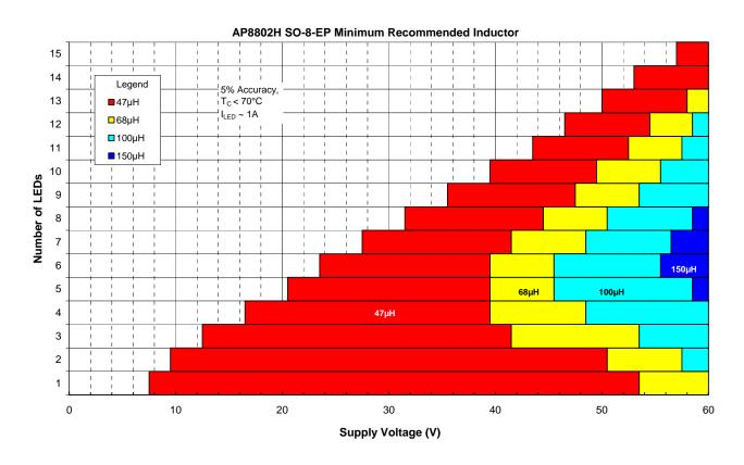
Figure 5: SO-8-EP recommended inductor with 1A LED current
