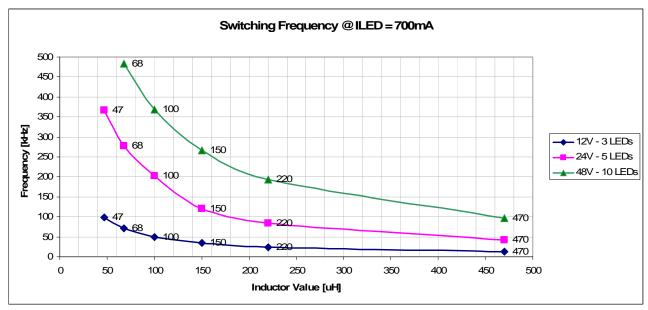
Figure 4: Switching Frequency Vs Inductor Value
