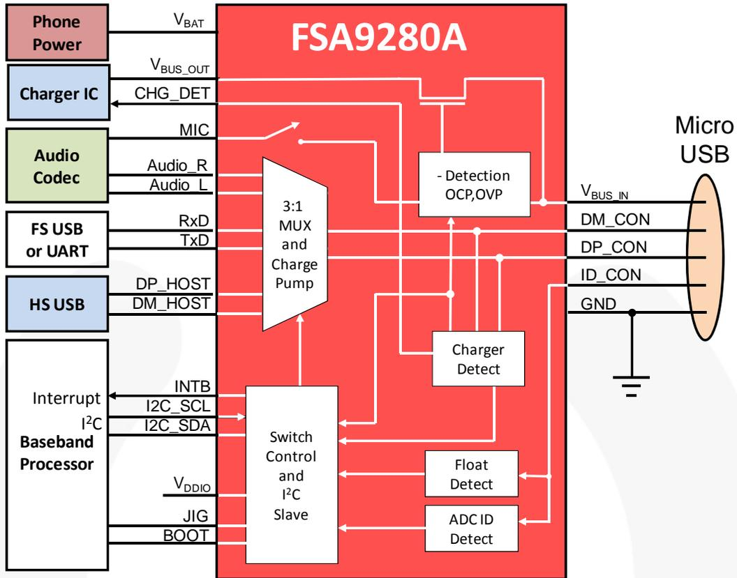
Figure 2. Block Diagram
