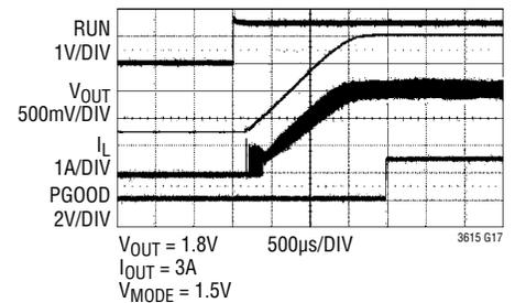
**TYPICAL PERFORMANCE CHARACTERISTICS**  $V_{IN} = 3.3V$ ,  $R_T/SYNC = SV_{IN}$ , unless otherwise noted.
