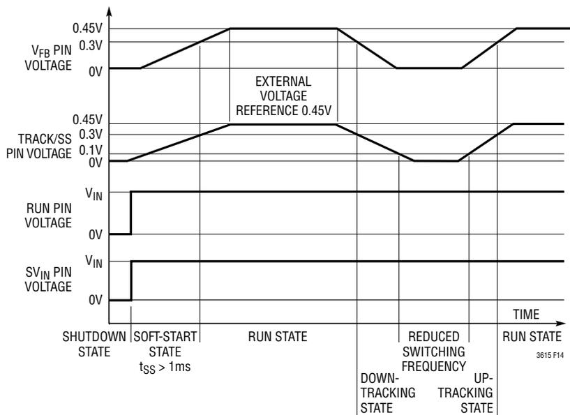
Figure 14. Tracking if  $V_{SRLIM}$  Is Tied to  $SV_{IN}$
