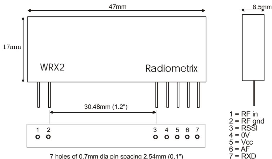
Figure 3: WRX2 pin-out and dimension (with can)
