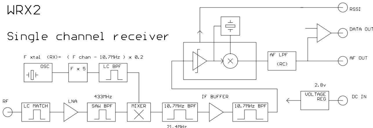
Figure 2: WRX2 block diagram
