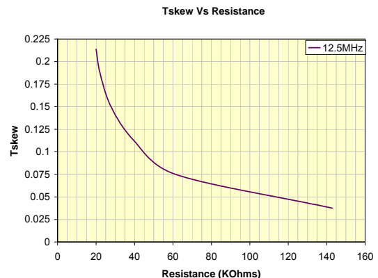
Fig10: Tskew Vs Resistance (12.5MHz, FS=1)
