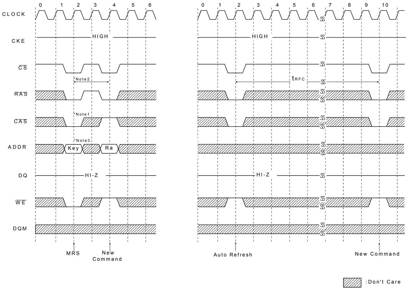
All banks precharge should be completed before Mode Register Set cycle and auto refresh cycle.
