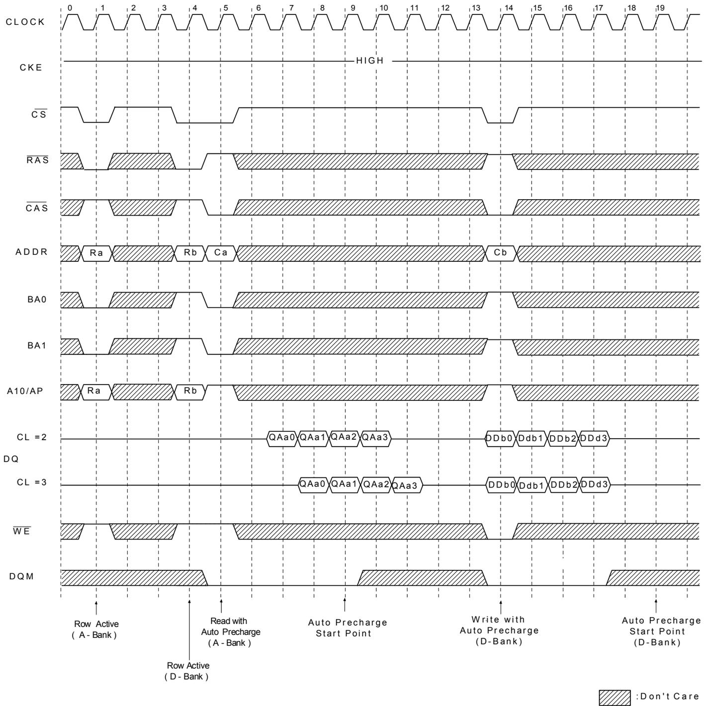
\*Note: 1.  $t_{CDL}$  should be controlled to meet minimum  $t_{RAS}$  before internal precharge start.
