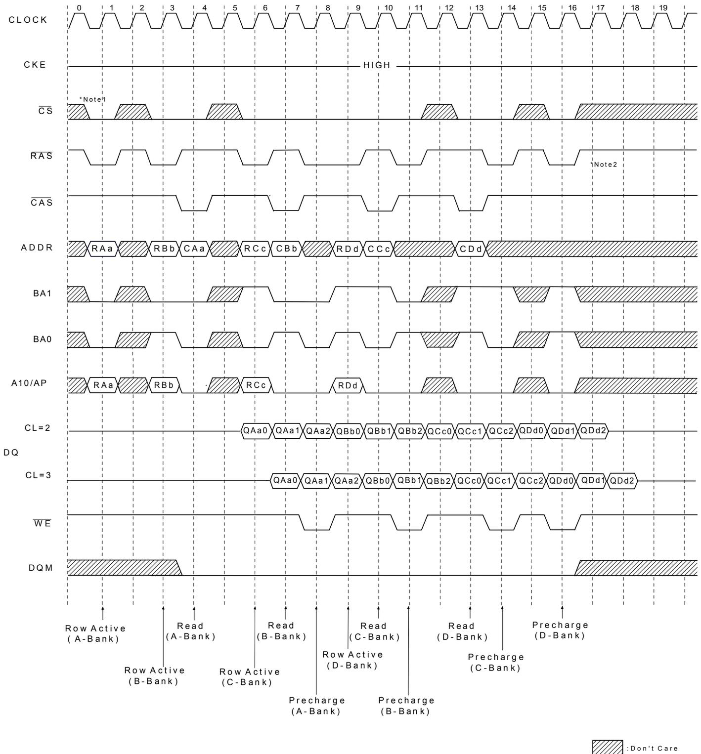
Note: 1.  $\overline{CS}$  can be don't cared when  $\overline{RAS}$ ,  $\overline{CAS}$  and  $\overline{WE}$  are high at the clock high going edge.
