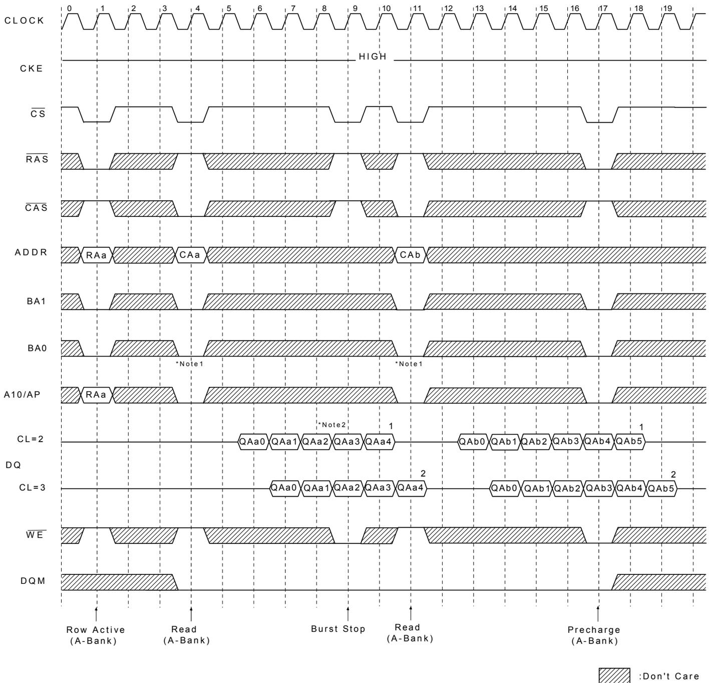
\*Note: 1. About the valid DQs after burst stop, it is same as the case of  $\overline{\text{RAS}}$  interrupt. Both cases are illustrated above timing diagram. See the table 1, 2 on them. But at burst write, Burst stop and  $\overline{\text{RAS}}$  interrupt should be compared carefully. Refer the timing diagram of "Full page write burst stop cycles".
