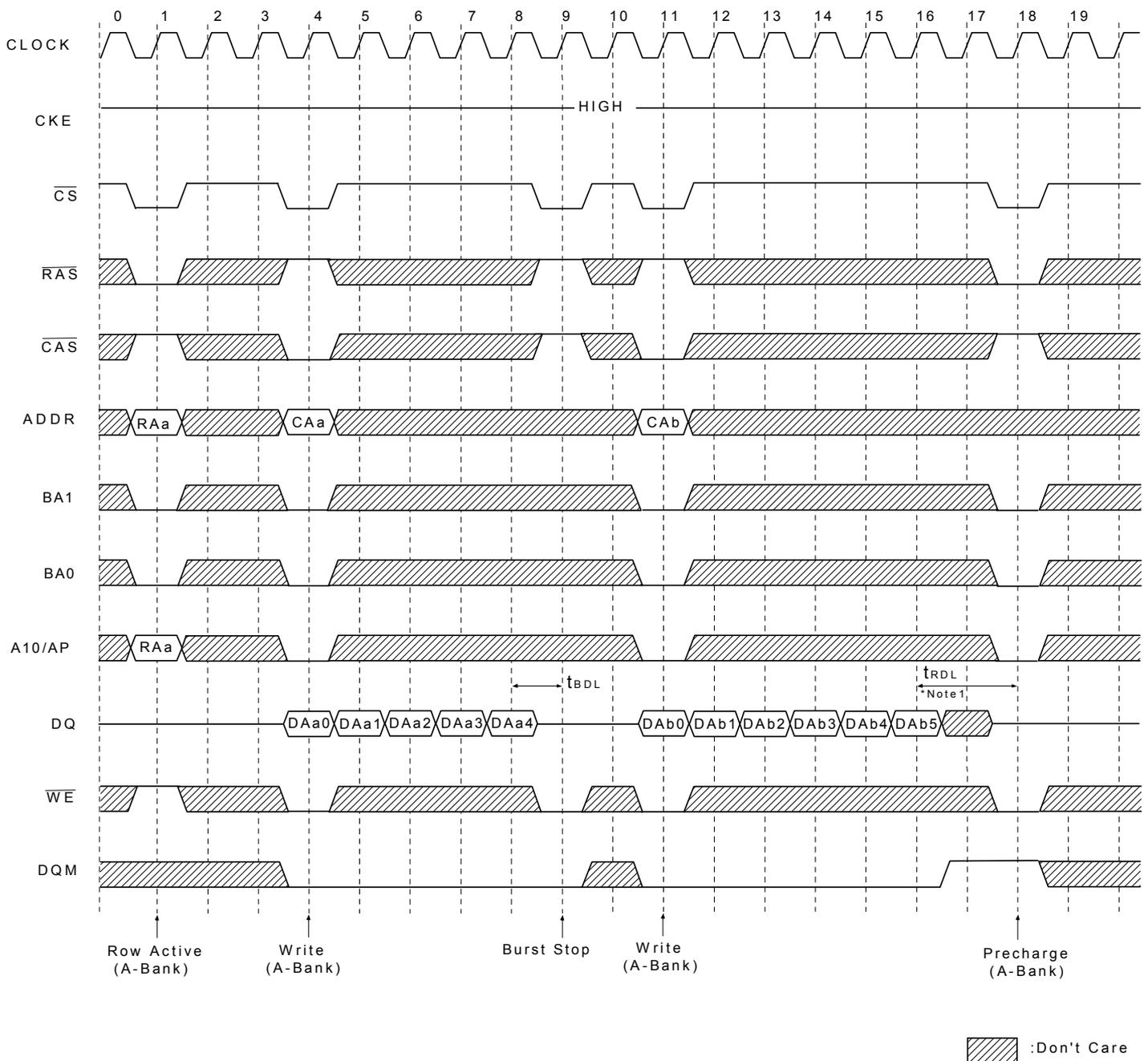
\*Note: 1. Data-in at the cycle of interrupted by precharge can not be written into the corresponding memory cell. It is defined by AC parameter of  $t_{RD1}$ .
