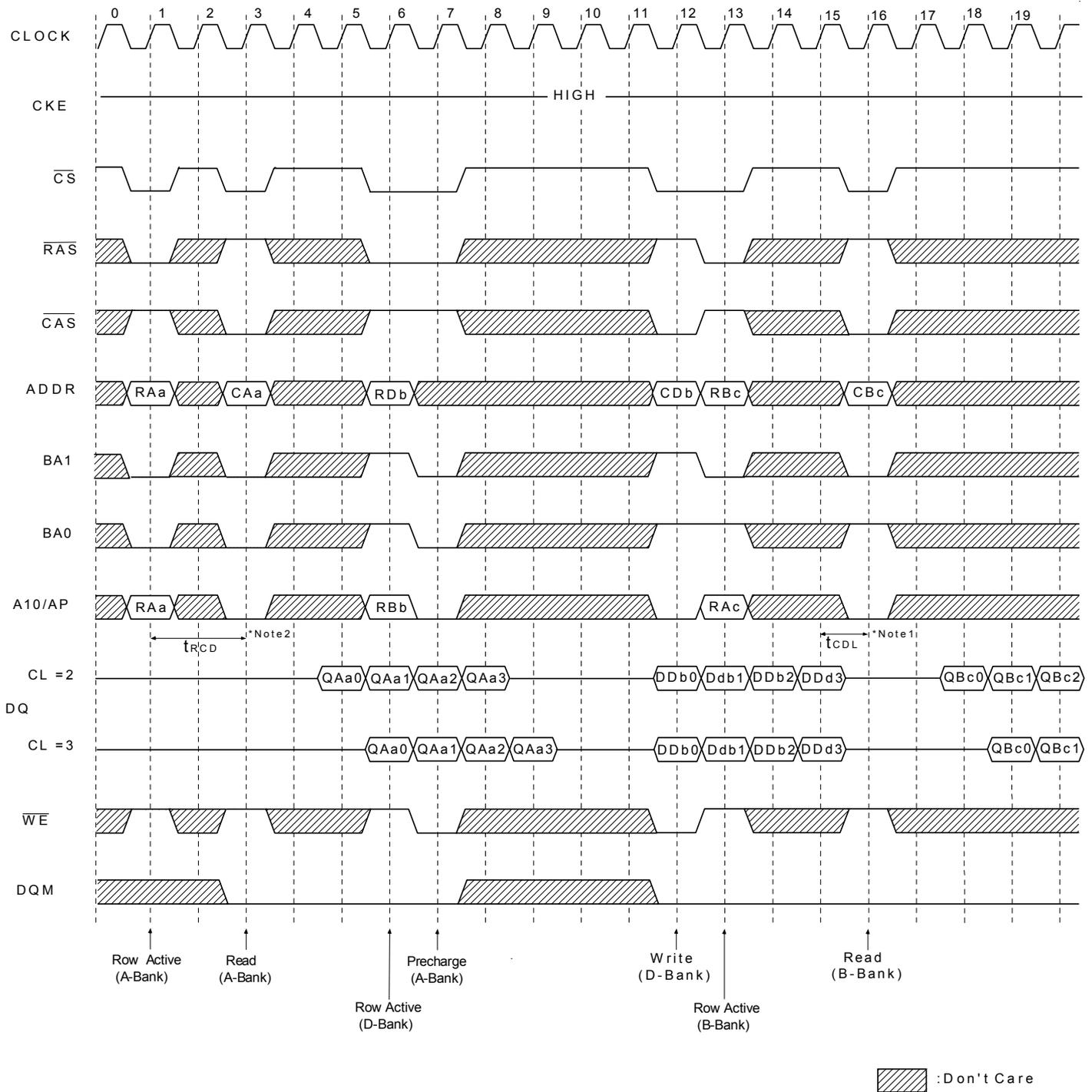
\*Note: 1.  $t_{CDL}$  should be met to complete write.
