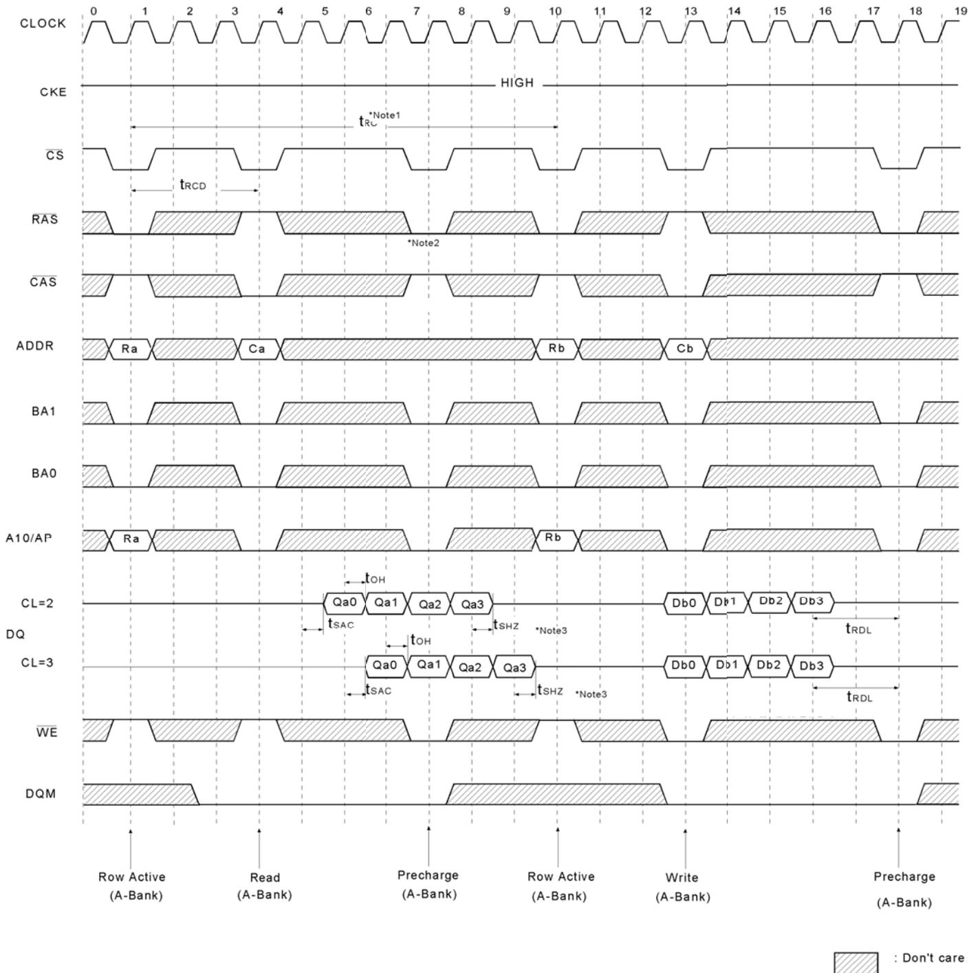
\*Note: 1. Minimum row cycle times is required to complete internal DRAM operation.
