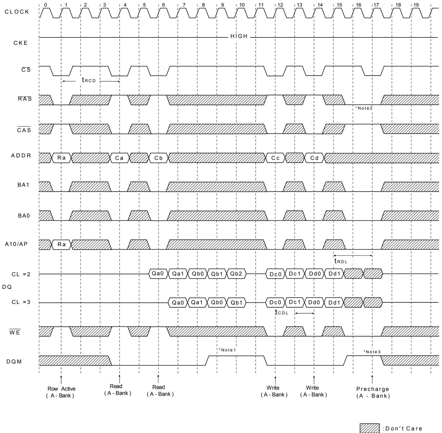
Note: 1. To Write data before burst read ends. DQM should be asserted three cycle prior to write command to avoid bus contention.
