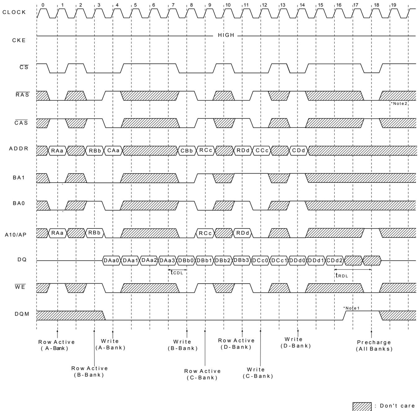
\*Note: 1. To interrupt burst write by Row precharge, DQM should be asserted to mask invalid input data.
