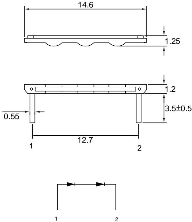
Note : 1.All dimension are in millimeter tolerance is  $\pm 0.25\text{mm}$  unless otherwise noted.
