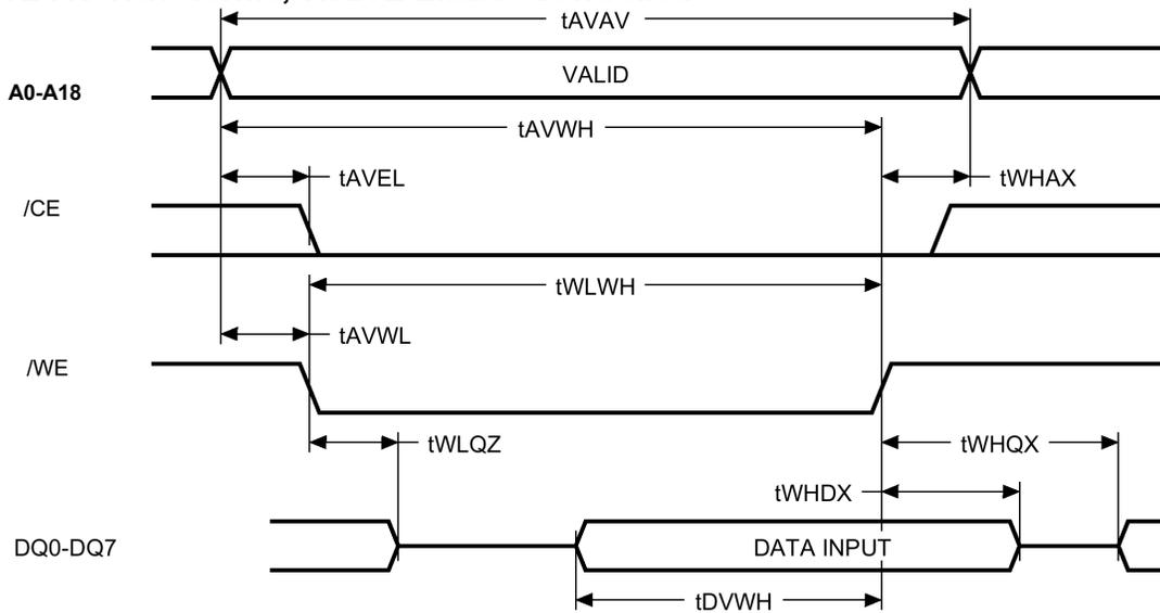
**WRITE AC Waveforms, Chip Enable Controlled**
