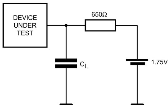
$C_L$  includes JIG capacitance
