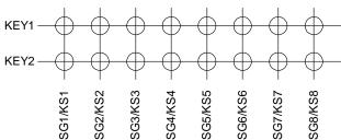
The data of each key is stored in key-input data RAM as illustrated below. They are read by a READ command, starting from the least significant bit. When the most significant bit of the data (SG8, b7) has been read, then the least significant bit of the next data (SGI, b0) will be read.
