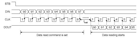
It must be noted that when the data is read, a waiting time  $t_{wait}$  of  $1\mu s$  is necessary between the rising of the eighth clock that has set the command and the falling of the first clock that has read the data.
