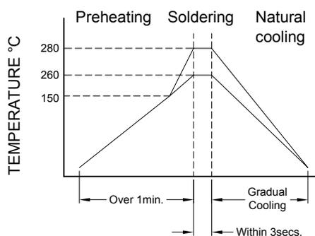
Figure 2. Iron Soldering
