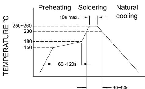
Figure 1. Re-flow Soldering
