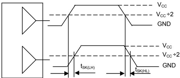
The pin-to-pin skew is defined as the worst case difference in propagation between any similar delay path within a single device
