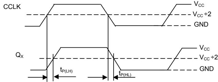
Figure 6. Propagation Delay ( $t_{PD}$ ) Test Reference
