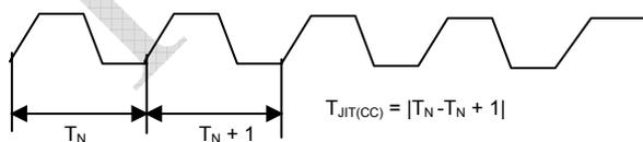
The variation in cycle time of a single between adjacent cycles, over a random sample of adjacent cycle pairs
