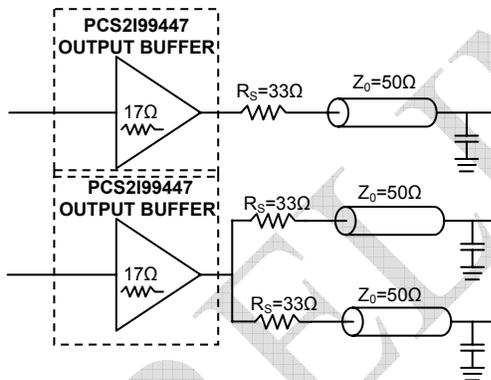
Figure 2. Single versus Dual Transmission Lines
