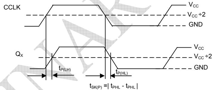
Figure 8. Output Pulse Skew ( $t_{SK(P)}$ ) Test
