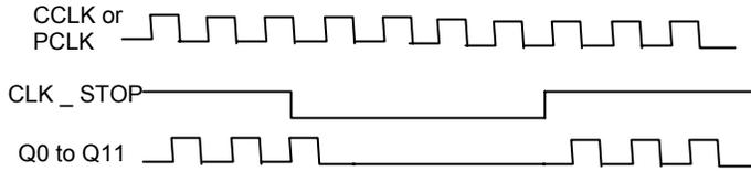
Figure 1. Output Clock Stop (CLK\_STOP) Timing Diagram
