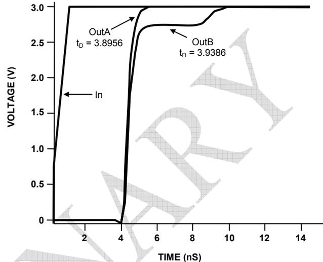
Figure 3. Single versus Dual Line Termination Waveforms
