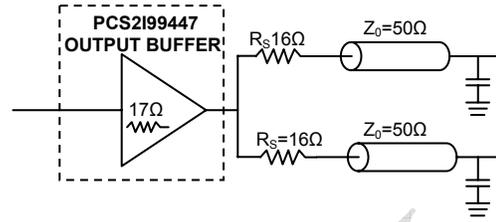
$$17\Omega + 16\Omega \parallel 16\Omega = 50\Omega \parallel 50\Omega$$
