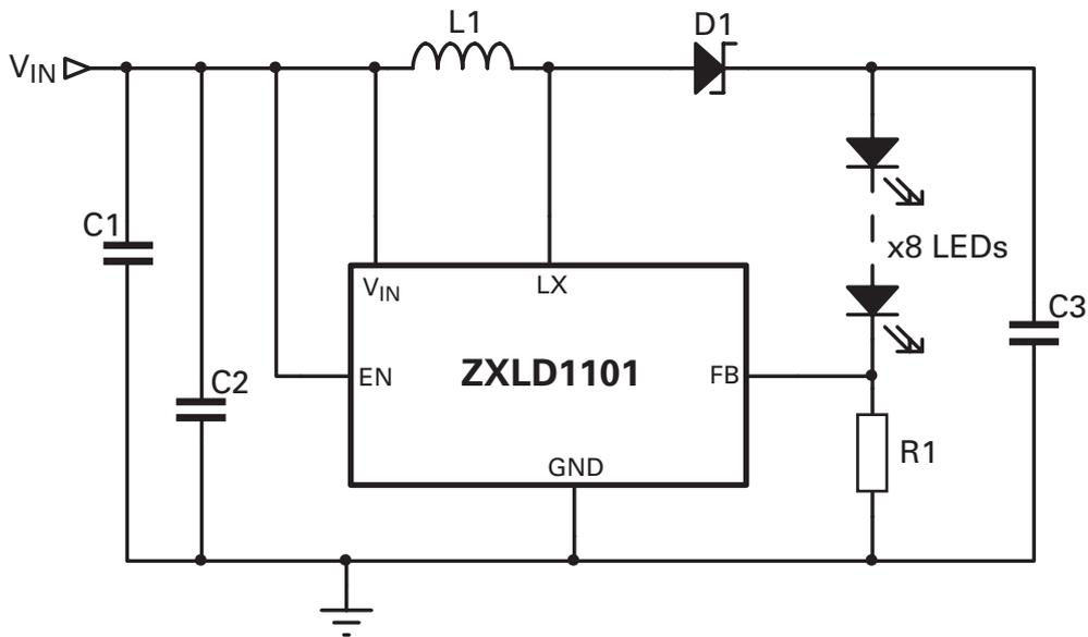
Figure 1 Schematic diagram
