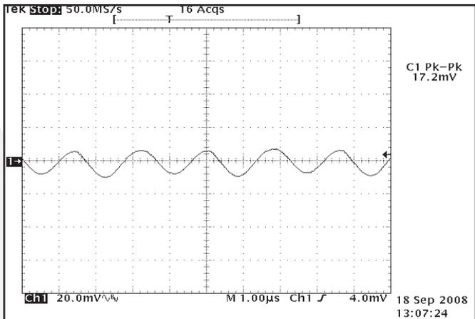
**Figure 16:** Output voltage ripple,  $V_{out}$ , at nominal input voltage and rated load current (20 mV/div). Load capacitance: 1 $\mu$ F ceramic capacitor and 10 $\mu$ F tantalum capacitor. Bandwidth: 10 MHz. See Figure 14.
