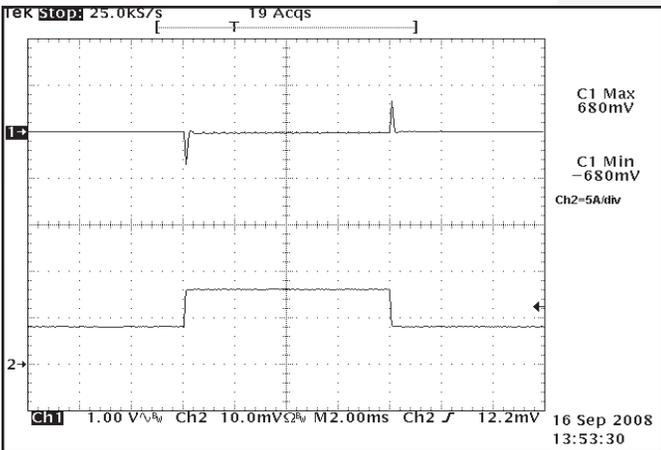
**Figure 11:** Output voltage response to step-change in load current 50%-100%-50% of Iout (max). Load cap: 1μF ceramic cap and 10μF, 100 mΩ ESR tantalum cap. Ch 1: Vout (1V/div). Ch 2: Iout (5A/div).
