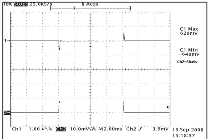
**Figure 12:** Output voltage response to step-change in load current 0%-50%-0% of Iout (max). Load cap: 1μF ceramic cap and 10μF, 100 mΩ ESR tantalum cap. Ch 1: Vout (1V/div). Ch 2: Iout (5A/div).
