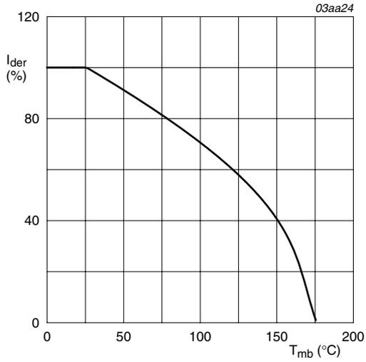
$$I_{der} = \frac{I_D}{I_{D(25^\circ\text{C})}} \times 100\%$$
