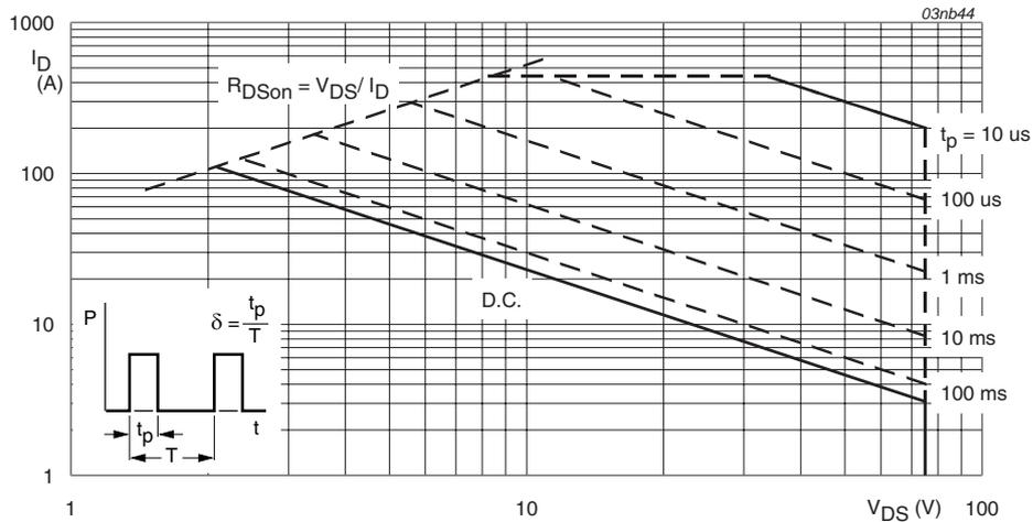
$T_{mb} = 25^\circ\text{C}; I_{DM}$  is single pulse
