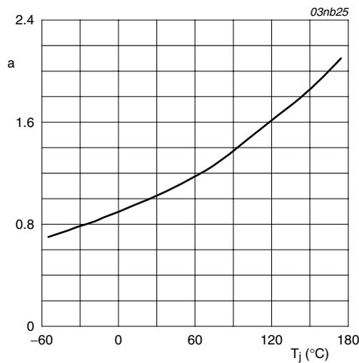
$$a = \frac{R_{DSon}}{R_{DSon(25^{\circ}C)}}$$
