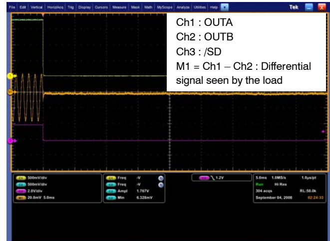
Figure 28. Zero pop noise turn off sequence with single-ended input audio source ( C_i = 100 nF, R_i = 24 k \Omega , R_f = 24 k \Omega , C_{byp} = 1 \mu F, R_L = 8 \Omega , T_{on} = GND )
