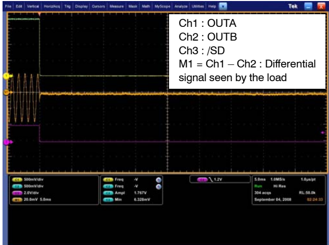
Figure 40. Zero pop noise turn off sequence with differential input audio source ( C_i = 47 \text{ nF} , R_i = 24 \text{ k}\Omega , R_f = 24 \text{ k}\Omega , C_{byp} = 1 \text{ }\mu\text{F} , R_l = 8 \text{ }\Omega , T_{on} = V_p )
