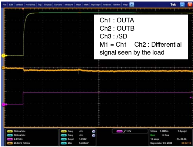
Figure 33. Zero pop noise turn on sequence with single-ended input to ground ( C_i = 47\text{ nF} , R_i = 24\text{ k}\Omega , R_f = 24\text{ k}\Omega , C_{byp} = 1\text{ }\mu\text{F} , R_l = 8\text{ }\Omega , T_{on} = V_p )
