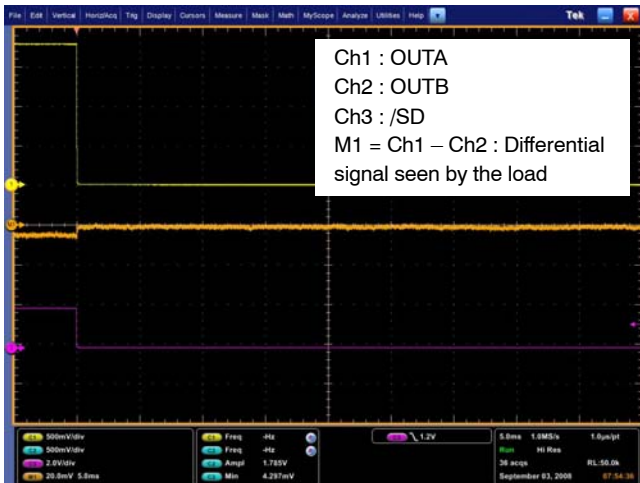
Figure 27. Zero pop noise turn off sequence with single-ended input to ground ( C_i = 100 nF, R_i = 24 k \Omega , R_f = 24 k \Omega , C_{byp} = 1 \mu F, R_L = 8 \Omega , T_{on} = GND )
