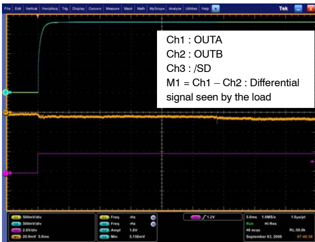
Figure 25. Zero pop noise turn on sequence with single-ended input to ground ( C_i = 100 nF, R_i = 24 k \Omega , R_f = 24 k \Omega , C_{byp} = 1 \mu F, R_L = 8 \Omega , T_{on} = GND )
