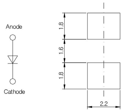
( Tolerance:  $\pm 0.2$ , Unit: mm )
