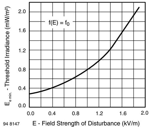
Fig. 8 - Sensitivity vs. Electric Field Disturbances
