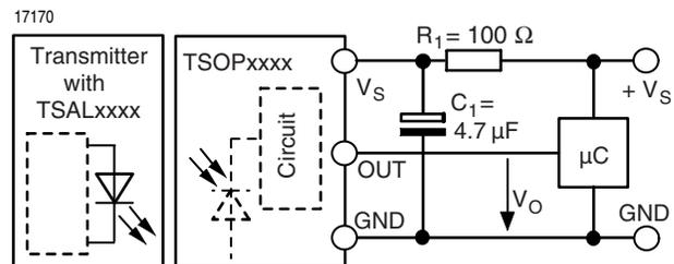
$R_1$  and  $C_1$  recommended to suppress power supply disturbances. The output voltage should not be hold continuously at a voltage below  $V_O = 2.0$  V by the external circuit.
