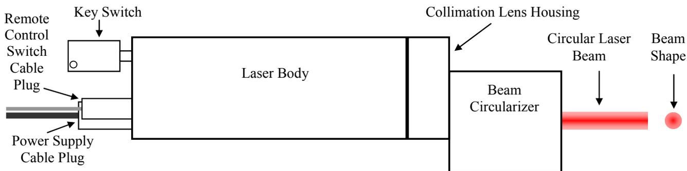
Figure 3 Generating a Circular Laser Beam
