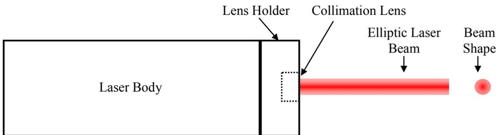
Figure 2B Generating a Circular Laser Beam by Using a Special Laser Diode
