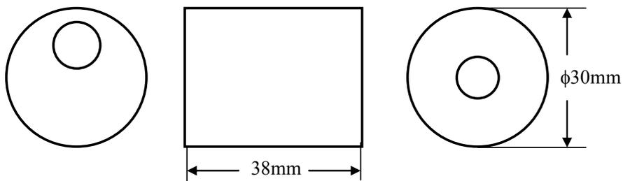
Figure 7 Beam Circularizer
