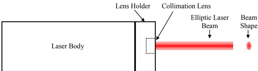
Figure 2A Generating an Elliptic Laser Beam
