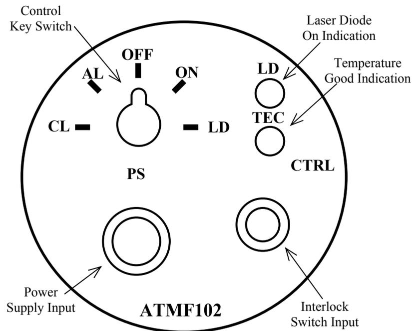
Figure 4 Back View of the Laser
