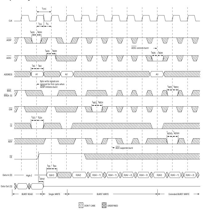
18. Full width Write can be initiated by either  $\overline{\text{GW}}$  LOW; or by  $\overline{\text{GW}}$  HIGH,  $\overline{\text{BWE}}$  LOW and  $\overline{\text{BW}}_{[A:D]}$  LOW.
