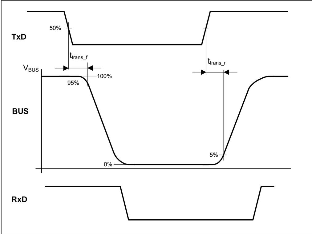
**Figure 2 – Transmit delay**
