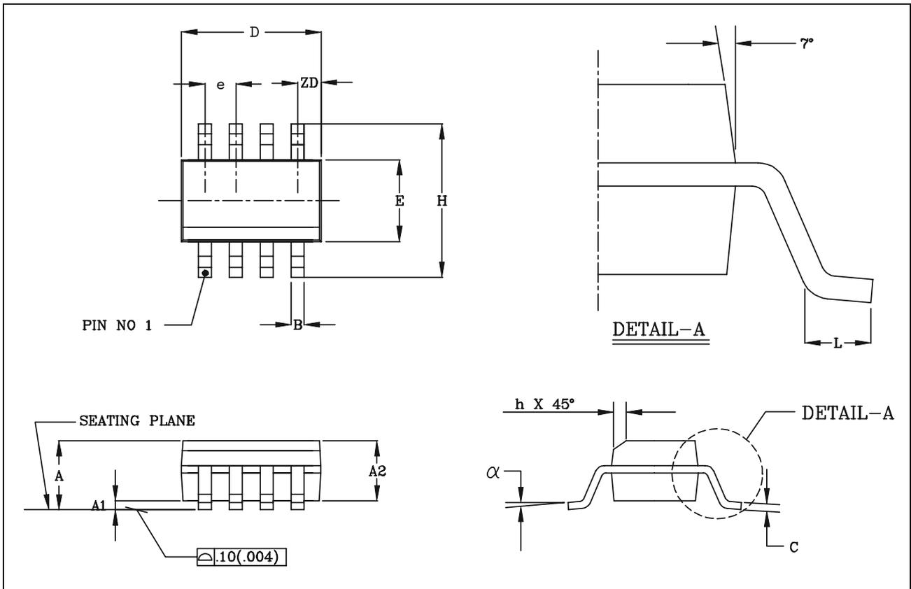
Small Outline Integrated Circuit (SOIC), SOIC 8, 150 mil
