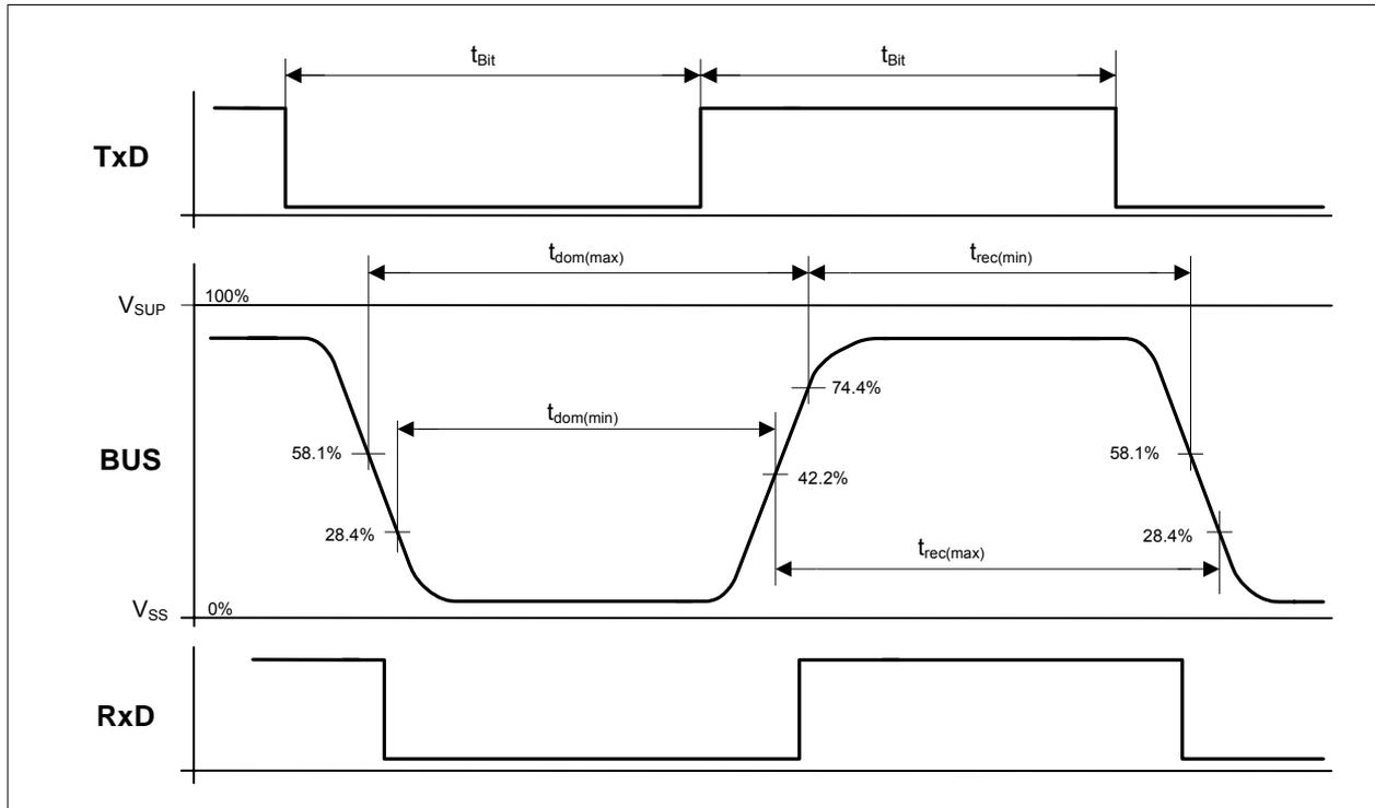
Figure 8 - Duty cycle calculation in accordance to LIN 2.0
