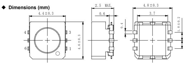
\* Dimension does not include solder used on coil.
