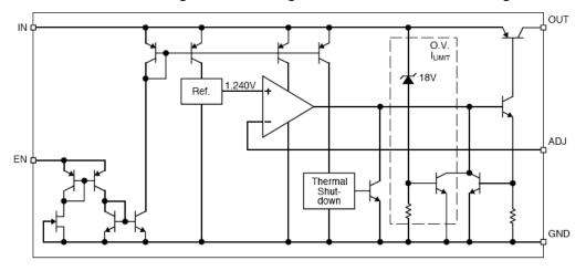
TS39152 Adjustable Regulator Block Diagram
