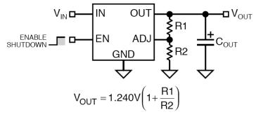
Where  $V_{OUT}$  is the desired output voltage. Above application circuit shows component definition. Applications with widely varying load currents may scale the resistors to draw the minimum load current required for proper operation.
