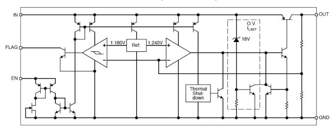
TS39151/3 Fixed Regulator with Flag, Sense and Enable Block Diagram
