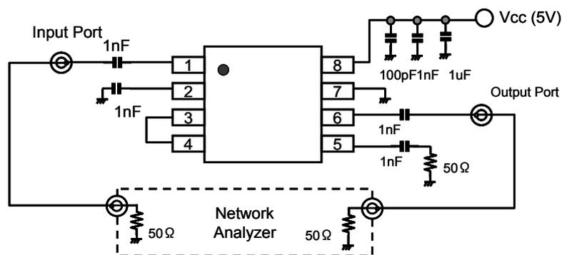
**Figure 4 Measurement circuit**
