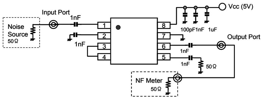
**Figure 3 Measurement circuit**
