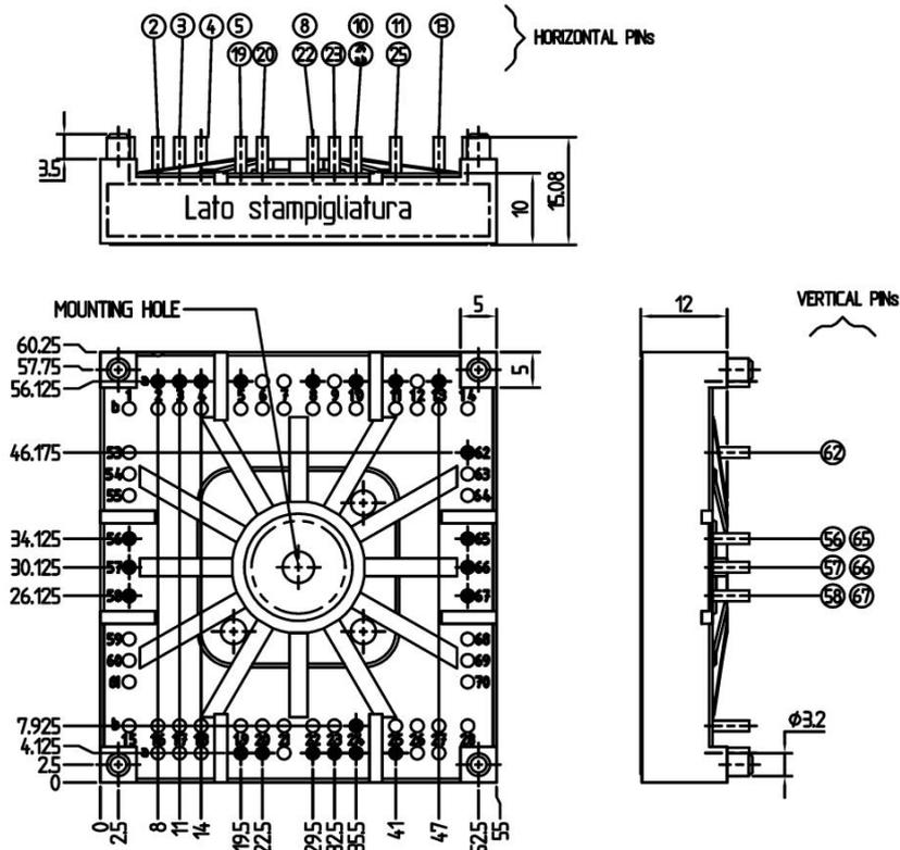
Case T74 (Suggested hole diameter for the solder pins in the circuit board: 2mm. Suggested hole diameter for the mounting pins in the circuit board: 3,6mm )
