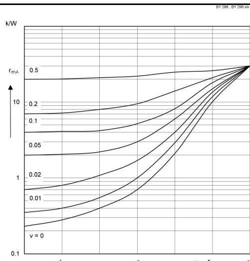
Fig. 3 Pulse thermal resistance vs. pulse duration <sup>1)</sup>
