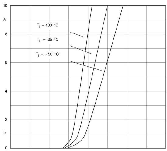
Fig. 1 Forward characteristic ( typical values )
