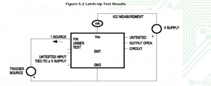
Test Circuit: Positive Input/Output Overvoltage/Overcurrent
