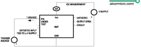
Test Circuit: Negative Input/Output Overvoltage/Overcurrent
