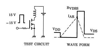
$$\begin{aligned} R_G &= 25~\Omega \\ V_{DD} &= 90~V,~L = 4.76~mH \end{aligned} \qquad E_{AS} &= \frac{1}{2} \cdot L \cdot I^2 \cdot \left( \frac{B_{VDSS}}{B_{VDSS} - V_{DD}} \right) \end{aligned}$$
