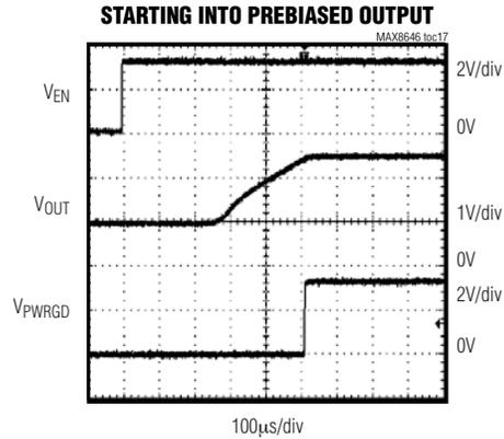
$C_{SS} = 6800pF$ ,  $C_O = 122\mu F$ ,  $L = 0.56\mu H$ ,  $V_{OUT} = 2.5V$
