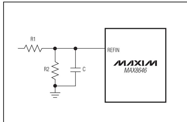
Figure 2. Typical Soft-Start Implementation with External Reference
