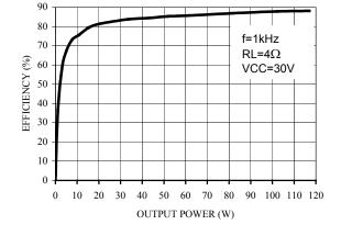
EFFICIENCY vs OUTPUT POWER (parallel operation)
