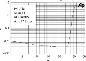
THD+N vs OUTPUT POWER (parallel operation) 10 Ap f=1kHz  $RL=4\Omega$ 1 VCC=30V AES17 Filter 11 % 0.1 1/ 0.01 0.001 2 5 20 50 1 10 100 200 W
